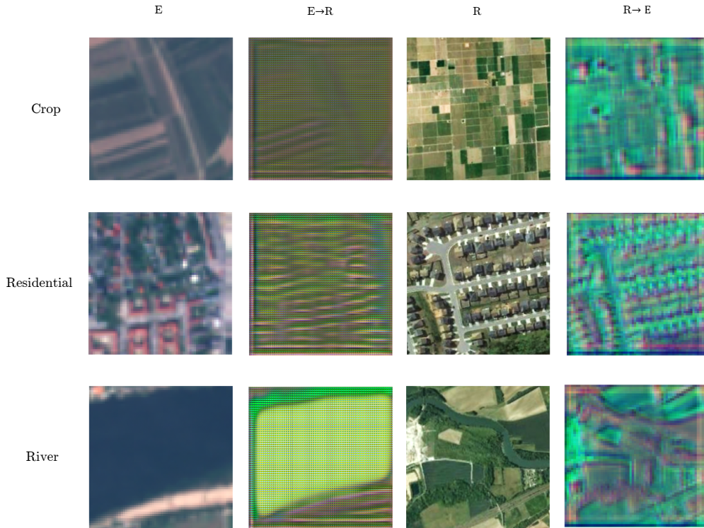
Figure 4.14: The translation of images with the semi-supervised CycleGAN for HDA using labelled RESISC45 as a source domain and the EuroSAT with 6.25% of the labelled data as a target domain. First column — original Eurosat images (E). Second column — Eurosat images translated to RESISC45 (E→R). Third column — original RESISC45 images (R). Fourth column — RESISC45 images translated to EuroSAT.
