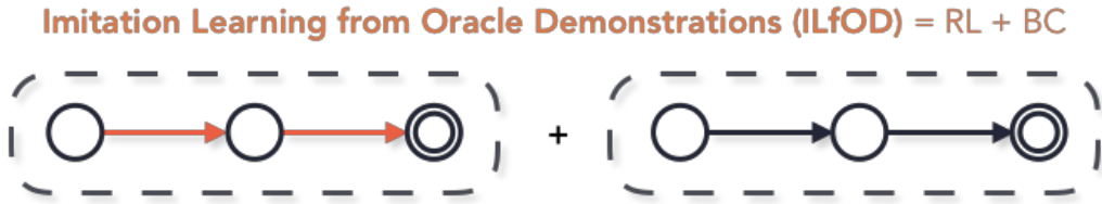
Figure 3.3: ILfOD is based on the experience replay composed of both oracle and agent trajectories (represented by two different datasets). The states are represented by circles (double circle for the terminal state), the oracle’s actions by orange arrows and the agent’s actions by black arrows.
