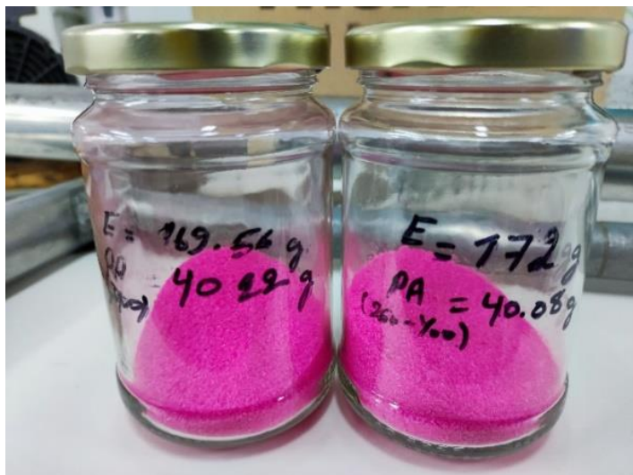
Supplementary Figure 2 Colored Polyamide fragments after being stained with Nile Red solution and oven-dried at 55 °C for 48 hours.
