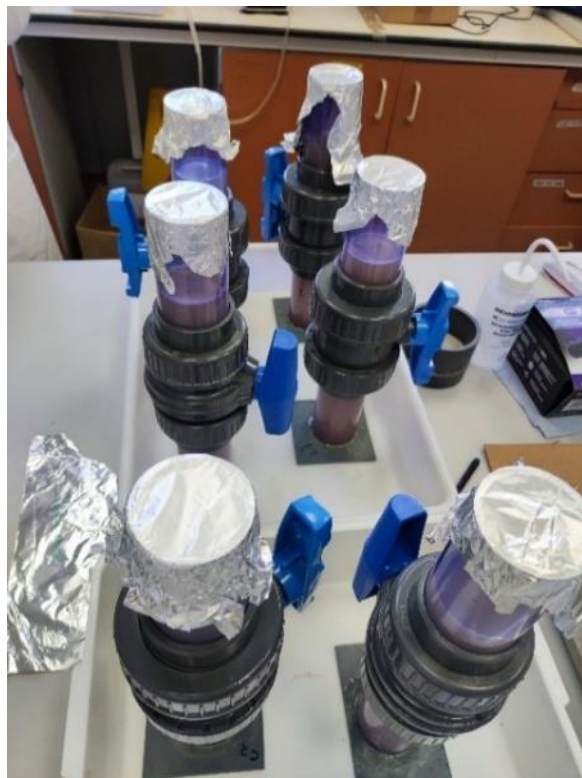
Supplementary Figure 4 Density separation of the polyamide fragments from sediments using Sediment Microplastic Isolation (SMI) units and zinc chloride ( \text{ZnCl}_2 ; 1.5 \text{ g cm}^{-3} ).
