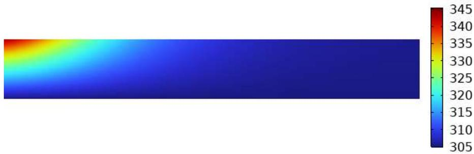
Figure 29. Temperature distribution in the anode at 10 s.
