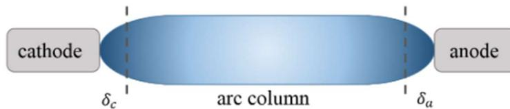
Figure 1. Schematic of the electric arc. Source: [5]
