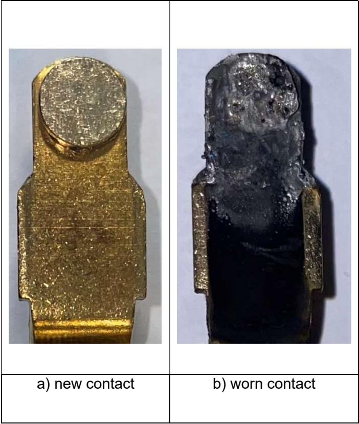
Figure 4. Comparison between a new electrical contact and a worn one. Source: [20].
