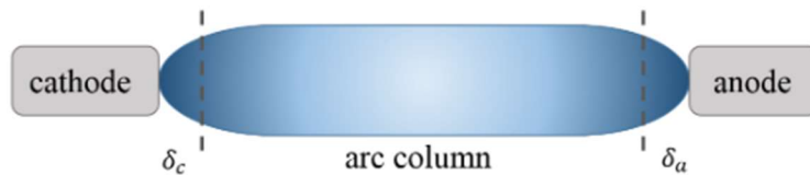
Figure 1. Schematic of the electric arc. Source: [5]
