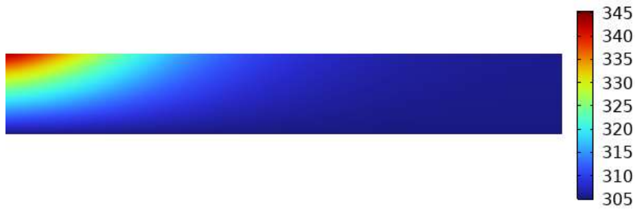
Figure 29. Temperature distribution in the anode at 10 s.
