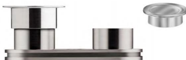
Figure II-18. Schematic representation of servo cell of DSC. Two sensors are involved to determine the heat flux of sample, the reference, and the sample sensor.
