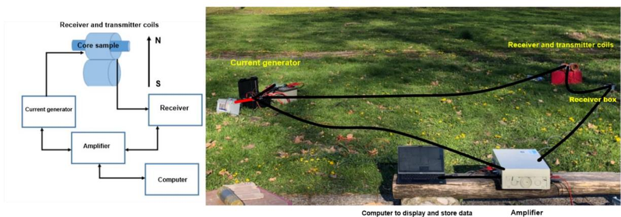
**Figure 3.29 Lab scale laboratory NMR instrument**
