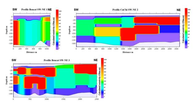
Figure 3 TDEM resistivity cross-section Ben Cat SW-NE1, SW-NE2, and SW-NE3
