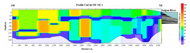
Figure 4.13 TDEM resistivity cross-section SW-NE1.
