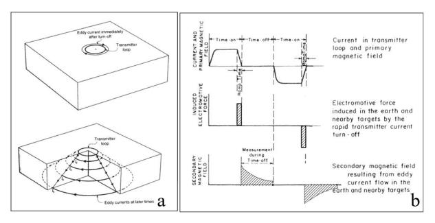
Figure 3.4 Illustration of the basic principles of the TDEM method (McNeill, 1994).
