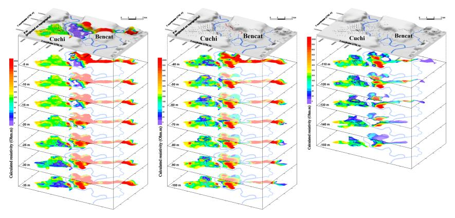
Figure 4.6 TDEM resistivity maps from 0 to -150m depth.
