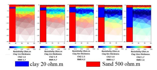
Figure 3.25 Inversion results showing variation in the thickness of clay within the synthetic model
