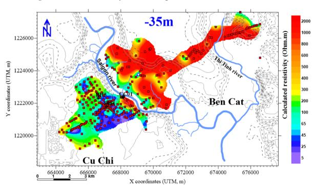
Figure 10 TDEM resistivity contour map at elevation -35m above sea level
