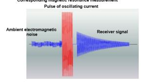
Figure 3.27 Typical phases of a magnetic resonance experiment.
