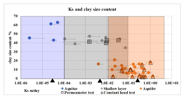
Figure 5.16 Correlation between saturated permeability and clay size content.
