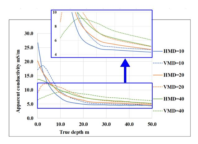
Figure 3.18 Comparison of synthetic apparent conductivity data of a 5-meter-thick clayey layer at different depths using VMD and HMD geometrical Tx-Rx configuration and using three Tx-Rx inter-coil spacings.
