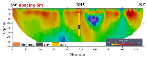
Figure 4.18 ERT results at BH5 with electrode spacing 5m
