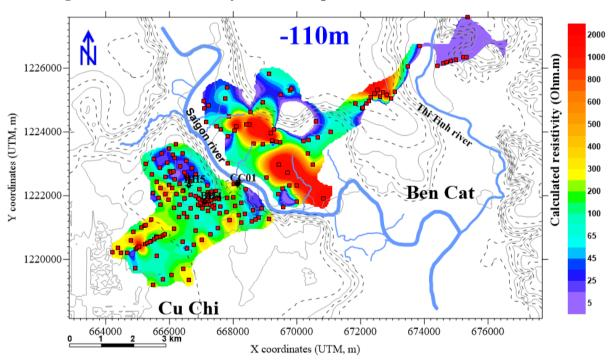
Figure 18TDEM resistivity contour map at elevation -110m above sea level
