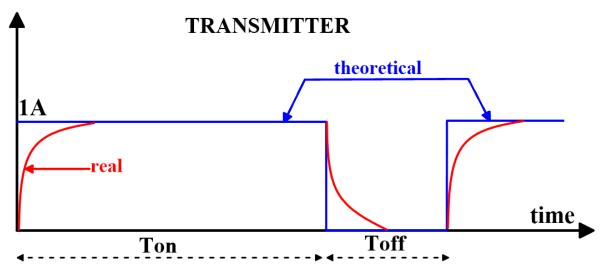
Figure 3.5 The pulses in a transmitter (AEMR technology).
