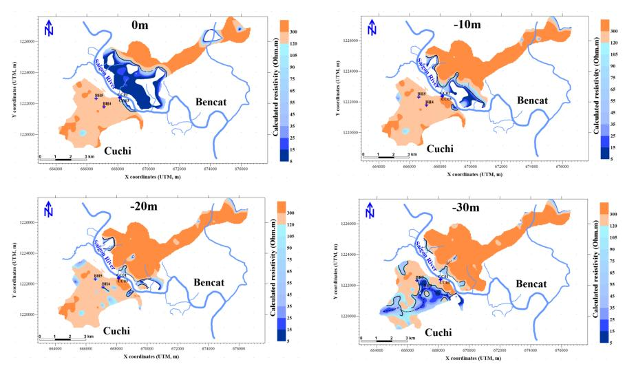
Figure 4.7 Resistivity contour maps at depth 0m, -10m, -20m and -30m with a simplified resistivity scale.
