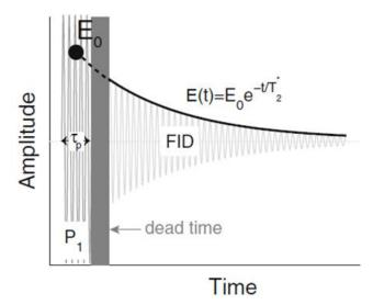
Figure 3.28 FID pulse sequence (Behroozmand, et al., 2015)
