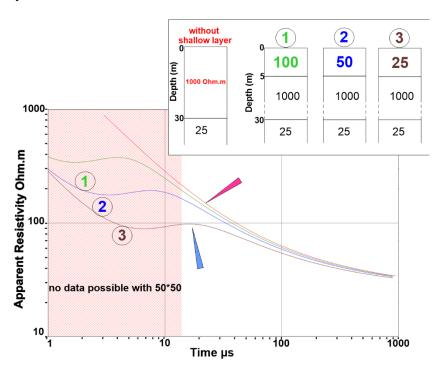
Figure 3.7 Apparent resistivity sounding curves from TDEM synthetic data.
