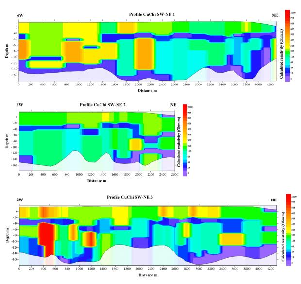
Figure 6 TDEM resistivity cross-section Cu Chi SW-NE1, SW-NE2 and SW-NE3
