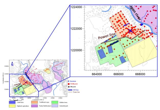
Figure 3.35 Study area with TDEM, ERT, and EM survey location.
