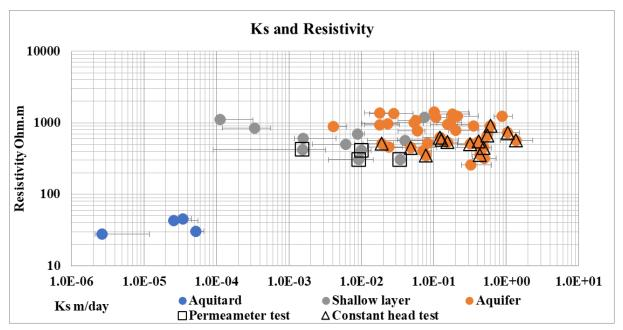
Figure 5.19 Correlation between saturated permeability and resistivity logging
