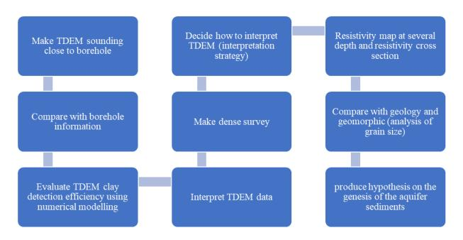
Figure 1.8 Overall methodology for applying Time-Domain Electromagnetic (TDEM) for aquifer geometry investigation.
