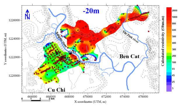
Figure 7 TDEM resistivity contour map at elevation -20m above sea level
