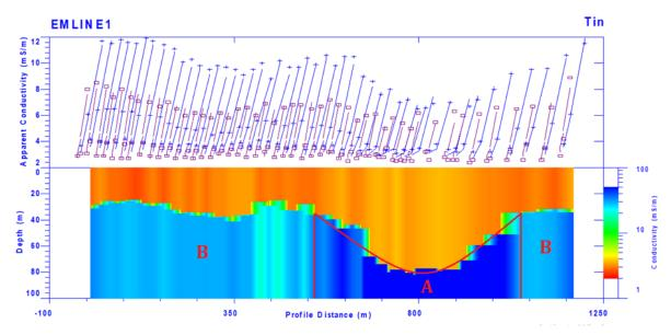
Figure 4.15 EM34 field data and interpreted result (2D model reconstructed from 1D interpretations) of EMLINE1 survey, respectively showing (A) the presence of "valley"; (B) shallower clay at roughly 30 meters.
