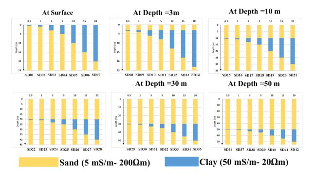
Figure 3.14 42 Synthetic model with different thicknesses and top depth of clay layer.
