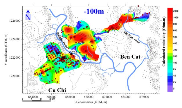
Figure 17 TDEM resistivity contour map at elevation -100m above sea level
