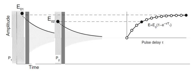
Figure 3.30 Saturation Recovery pulse sequence. The measurement initiates with a single 90° energizing pulse, denoted as P1, resulting in a corresponding Free Induction Decay (FID1).
