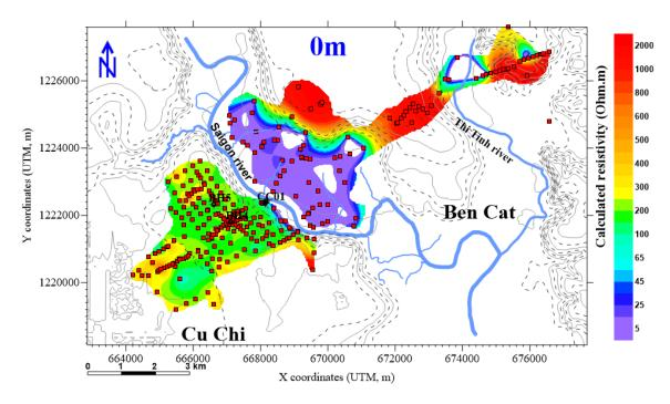
Figure 4.2 TDEM resistivity contour map at elevation 0m.
