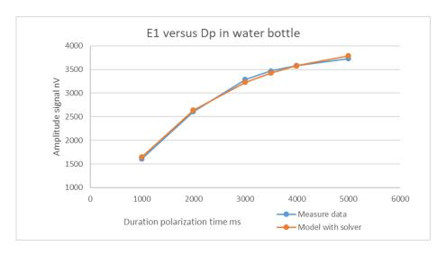
Figure 3.33 Amplitude versus duration polarization time for a bottle of water
