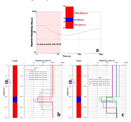
Figure 3.9 Synthetic model and interpretation result with equivalent models.
