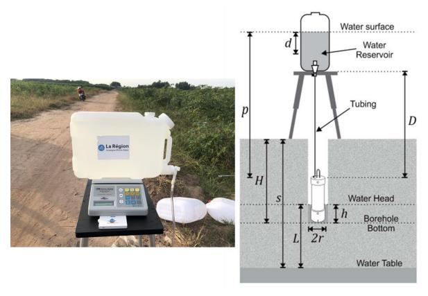
Figure 5.15 Permeameter test at the field BH4 site.
