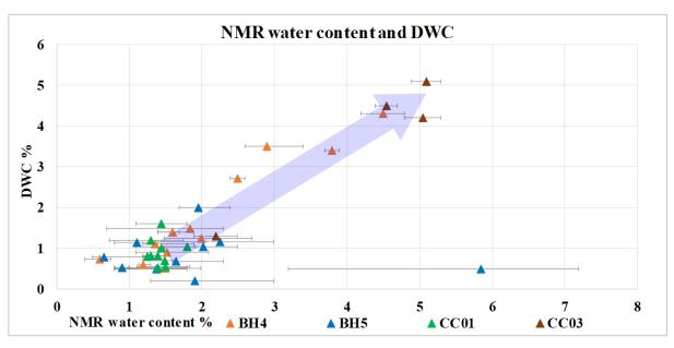
Figure 5.33 Relationship between NMR water content and drainage water content (DWC)
