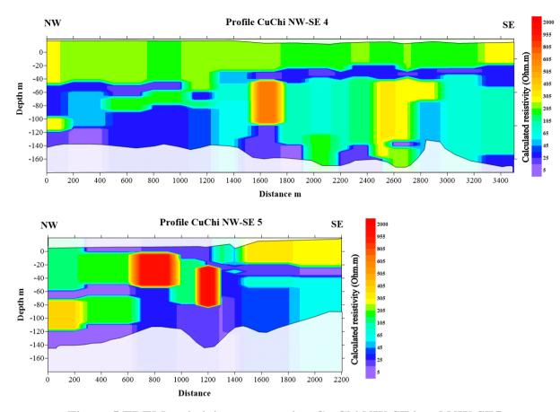
Figure 5 TDEM resistivity cross-section Cu Chi NW-SE4 and NW-SE5
