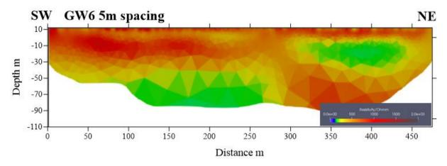
Figure 4 ERT profile at GW6 with 5m spacing
