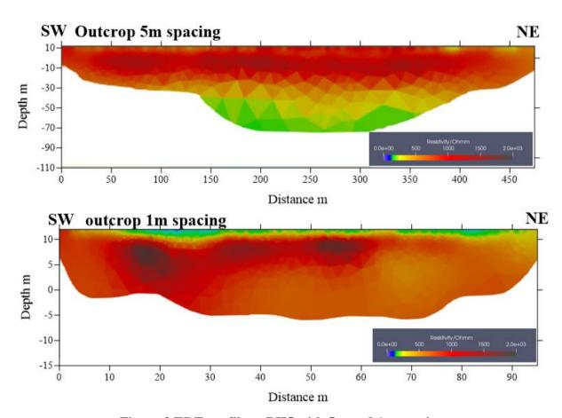
Figure 3 ERT profile at BH5 with 5m and 1m spacing
