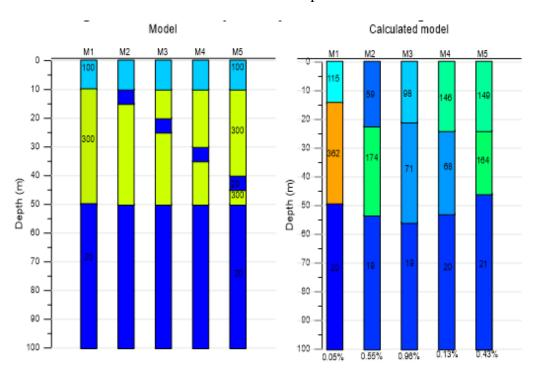
Figure 3.8 Compare resistivity values in the synthetic model and calculated model.
