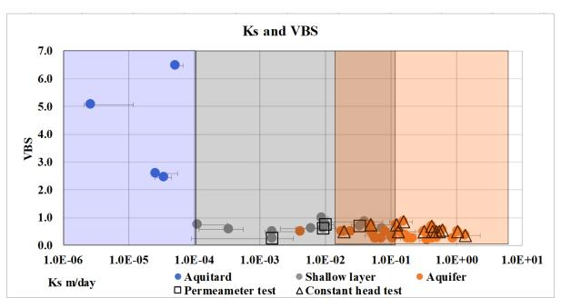
Figure 5.17 Correlation between saturated permeability and clay size content estimated by the VBS value obtained with the methylene blue test
