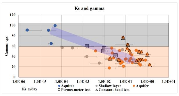
Figure 5.18 Correlation between saturated permeability (m/day) and gamma-ray (in count per second)
