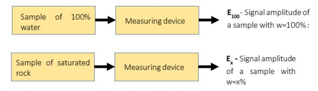
Figure 3.31 Procedure to measure the water content (Legchenko, 2022)
