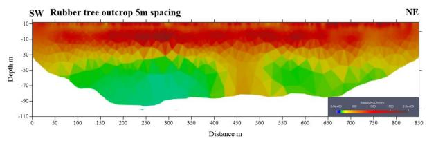
Figure 4.21 ERT results at" rubber tree" site with electrode spacing 5m
