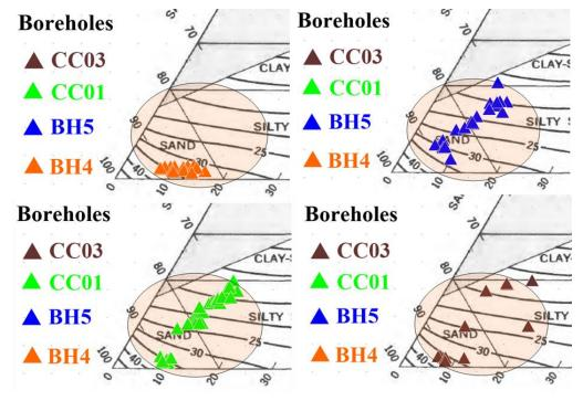
Figure 5.11 The classified specific yield (Sy) at CC01, CC03, BH4, and BH5 for the aquifer layer.
