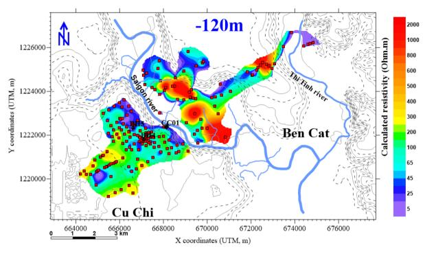
Figure 19 TDEM resistivity contour map at elevation -120m above sea level
