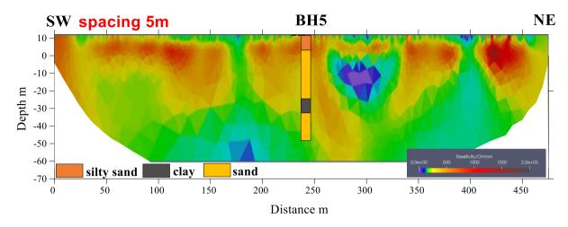
Figure 2 ERT profile at BH5 with 5m spacing
