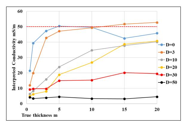
Figure 3.19 Comparison between the interpreted conductivity and true conductivity of clayey layer at different thicknesses and true depth of the top of the clayey layer.
