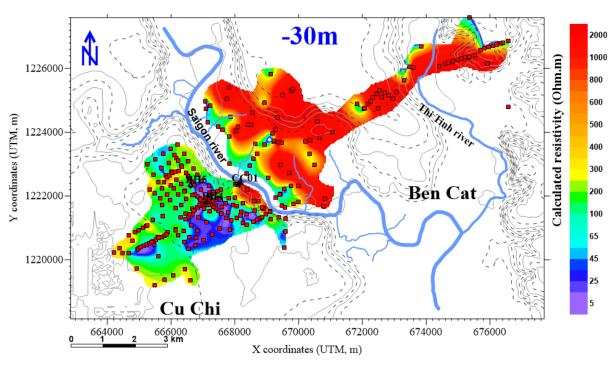
Figure 4.3 TDEM resistivity contour map at depth -30m below sea level.
