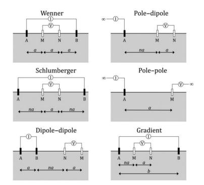
Figure 3.22 The main electrode configurations (Reynolds, 2011).
