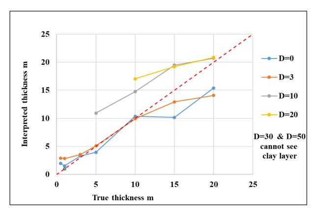
Figure 3.16 Comparison of true thickness and interpreted thickness of clay layer with EM34.
