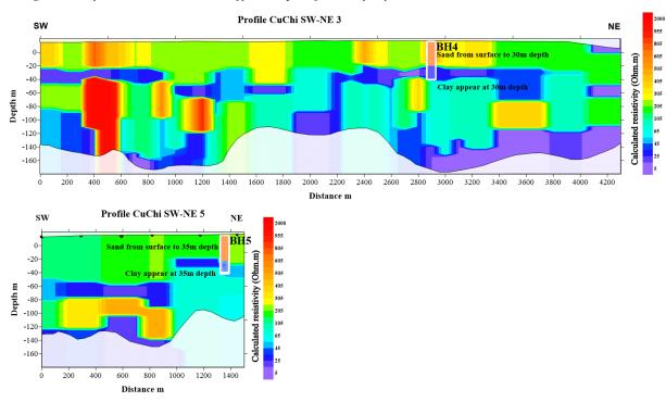
Figure 4.12 TDEM resistivity cross-section CC SW-NE3 and SW-NE5.
