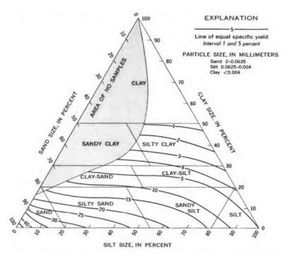
Figure 5.9 Soil classification triangle that illustrates the correlation between particle size distribution and specific yield (Johnson 1967)
