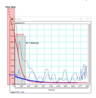
Figure 3.32 T2\* and extrapolation of the signal to 20ms delay time before
