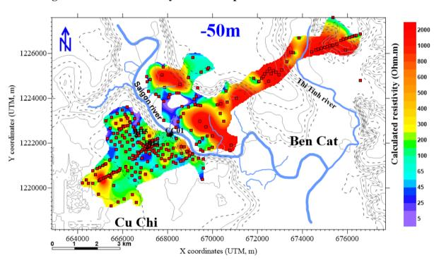
Figure 12 TDEM resistivity contour map at elevation -50m above sea level
