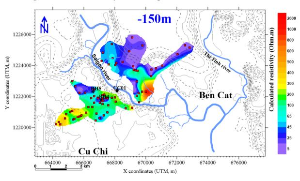
Figure 22 TDEM resistivity contour map at elevation -150m above sea level
