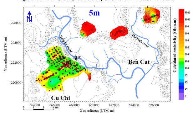
Figure 2 TDEM resistivity contour map at elevation +5m above sea level
