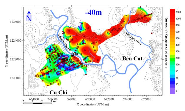
Figure 11 TDEM resistivity contour map at elevation -40m above sea level
