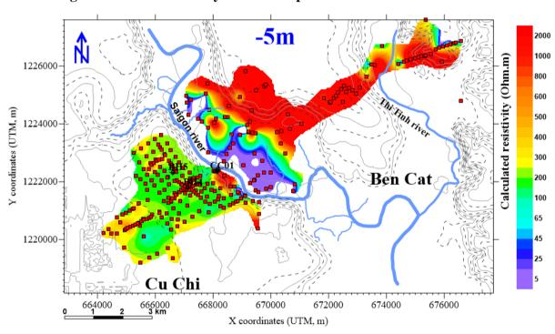
Figure 4 TDEM resistivity contour map at elevation -5m above sea level
