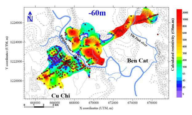
Figure 13 TDEM resistivity contour map at elevation -60m above sea level
