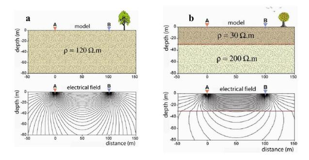
Figure 3.21 Current flow in the subsurface.
