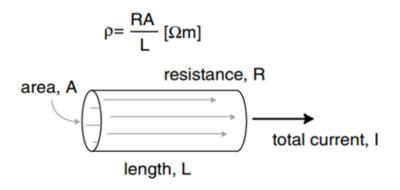
Figure 3.1 Parameters used in defining resistivity.
