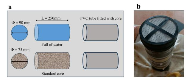
Figure 5.20 a) core sample and water sample tubes, b) Core sample after preparation before saturation step
