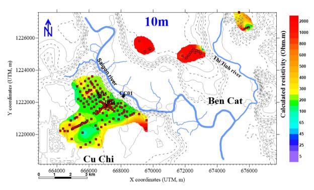
Figure 1 TDEM resistivity contour map at elevation +10m above sea level
