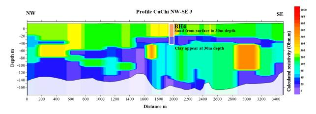
Figure 4.11 TDEM resistivity cross-section CC NW-SE3.
