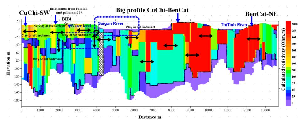
Figure 1 TDEM resistivity long profile
