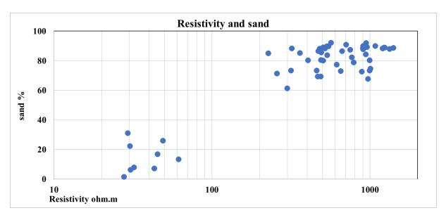
Figure 4.30 Correlation between well-log resistivity and the percentage of sand size in core samples
