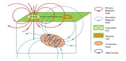
Figure 3.13 The FEM principles are applied to analyze the magnetic field response within a homogeneous half-space, considering the presence of a conductive body, transmitter, and receiver. (Reynolds, 2011).
