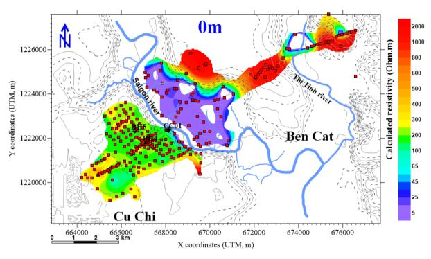
Figure 3 TDEM resistivity contour map at elevation 0m above sea level
