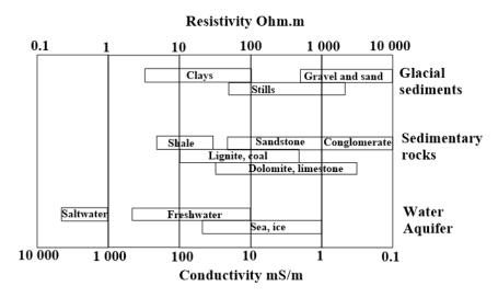
Figure 3.3 Typical ranges of electrical resistivity of earth material modified from (Palacky, 1987).
