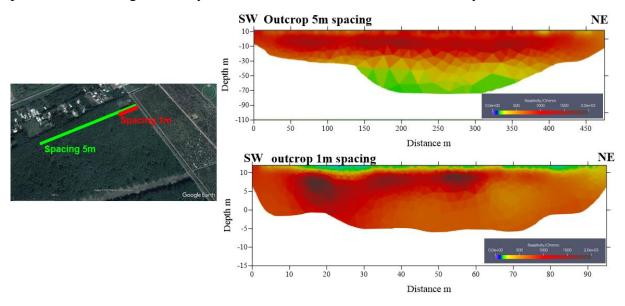
Figure 4.19 ERT results at outcrop site with electrode spacing 5m and 1m.
