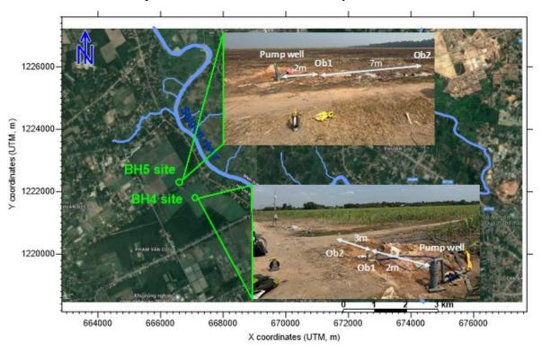
Figure 5.36 Location of pumping and tracer tests.
