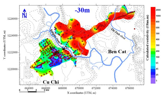
Figure 9 TDEM resistivity contour map at elevation -30m above sea level
