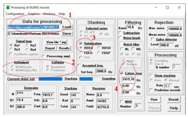
Figure 5.21 NUMIS PROGRAM for optimization, filtering, and stacking data before inversion.
