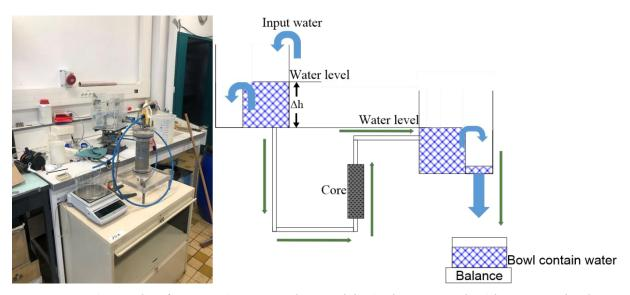
Figure 5.13 Procedure for measuring saturated permeability in the core sample with a constant head.
