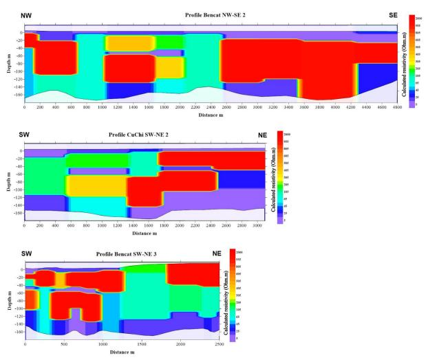
Figure 4.14 TDEM resistivity cross-section BC NW-SE2, BC SW-NE2 and BC SW-NE3.
