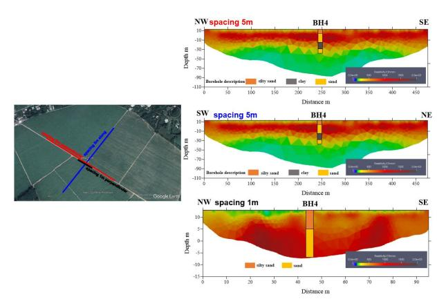
Figure 4.17 ERT results at BH4 with electrode spacing 5m to 1m.
