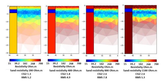
Figure 3.26 Inversion results showing Variation in the resistivity of the sand layer within the synthetic model
