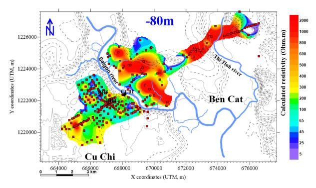
Figure 15 TDEM resistivity contour map at elevation -80m above sea level
