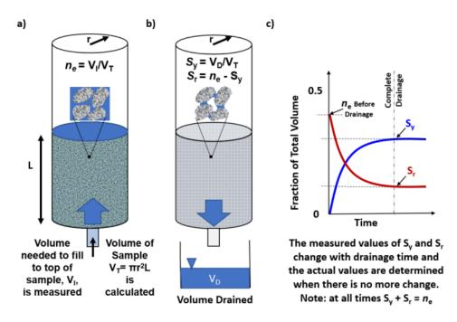
Figure 5.8 The determination of effective porosity (ne), specific yield (Sy), and specific retention (Sr) involves a multi-step process:
