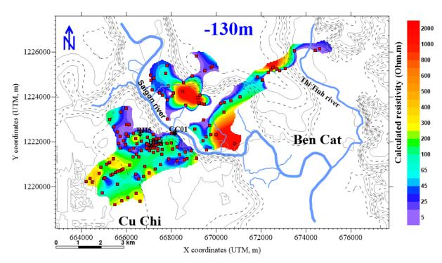
Figure 4.5 TDEM resistivity contour map at depth -130m bsl.
