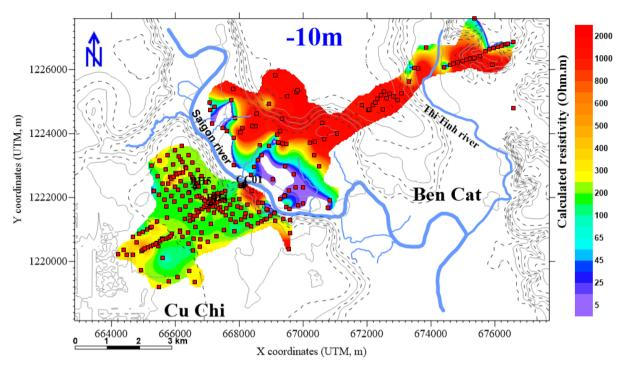
Figure 5 TDEM resistivity contour map at elevation -10m above sea level
