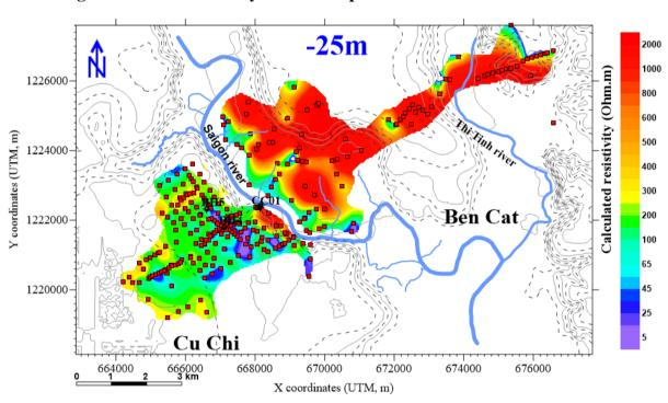
Figure 8 TDEM resistivity contour map at elevation -25m above sea level
