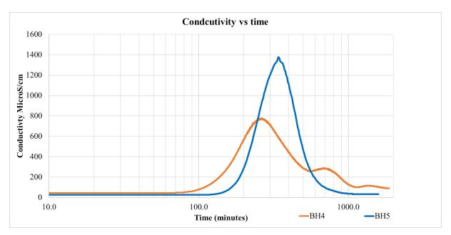
Figure 5.39 Electrical conductivity monitoring of water in the pumping wells.
