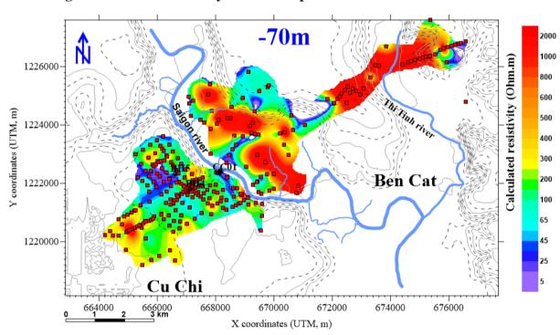
Figure 14 TDEM resistivity contour map at elevation -70m above sea level
