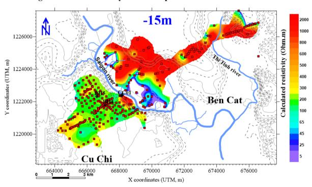
Figure 6 TDEM resistivity contour map at elevation -15m above sea level
