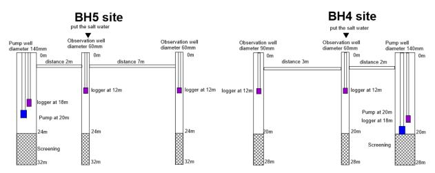
Figure 5.37 Well structure for pumping and tracer tests.
