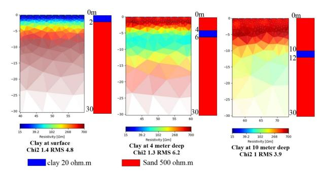
Figure 3.24 Inversion results showing variations in the depth of clay within the synthetic model.
