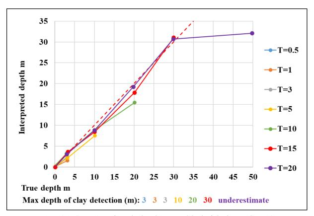
Figure 3.17 Comparison of true depth and interpreted depth of clay layer with EM34.
