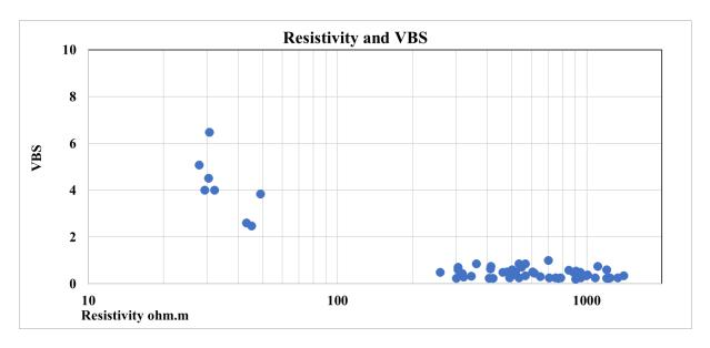
Figure 4.29 Relationship between well log resistivity and the VBS value obtained from the Methylene Blue experiment.
