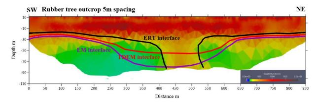
Figure 4.22 Comparison of resistivity results between EM34, TDEM and ERT at rubber tree outcrop. EM34 (purple), TDEM (red), ERT (black)
