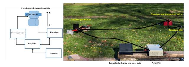
Figure 3.29 Lab scale laboratory NMR instrument
