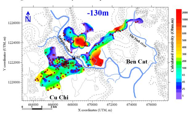
Figure 20 TDEM resistivity contour map at elevation -130m above sea level
