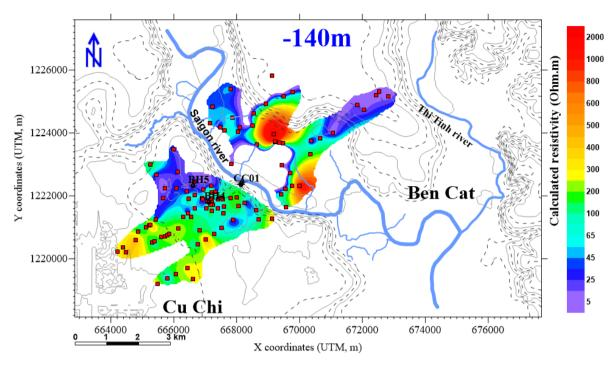
Figure 21 TDEM resistivity contour map at elevation -140m above sea level
