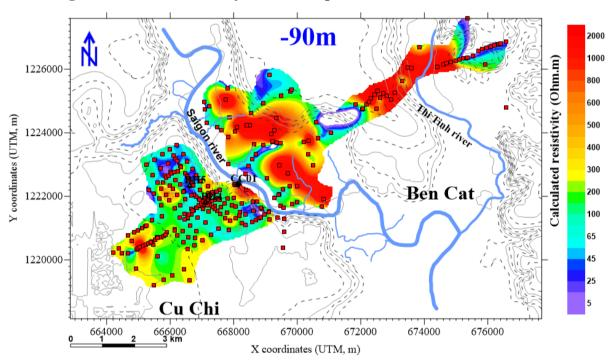
Figure 16 TDEM resistivity contour map at elevation -90m above sea level
