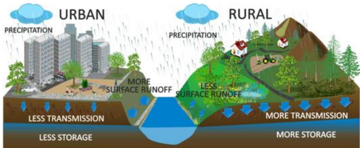
Figure 1.5 Simplified view of hydrological processes showing the main difference between urban and rural catchments.
