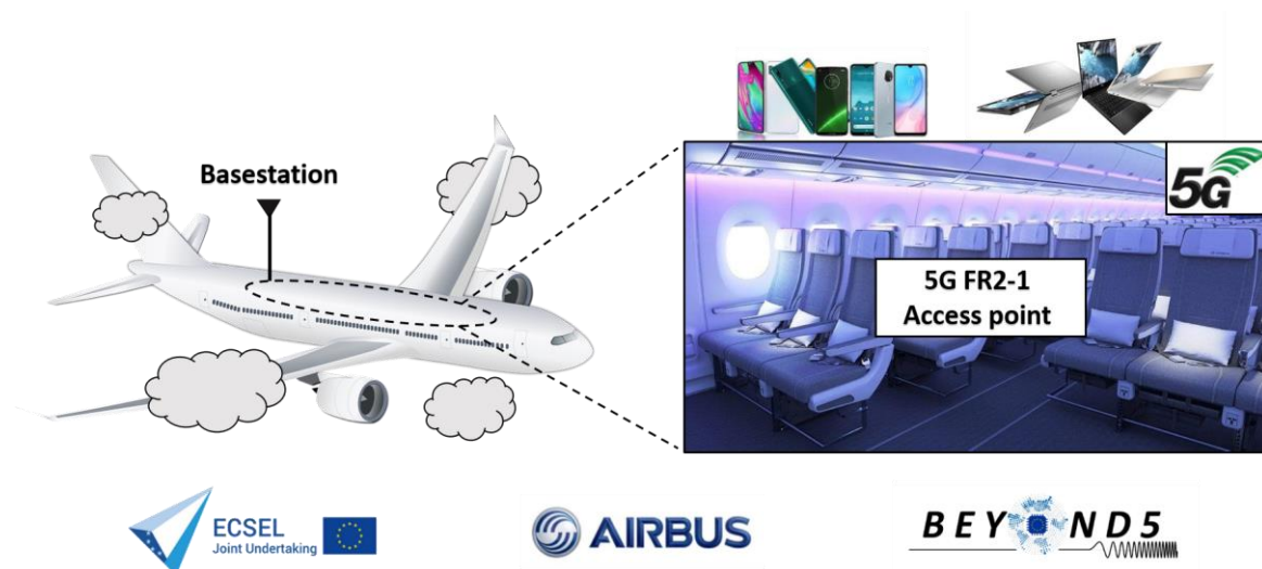
Figure 23: Illustration of the integration of a 5G FR2-1 MIMO on-flight access point
