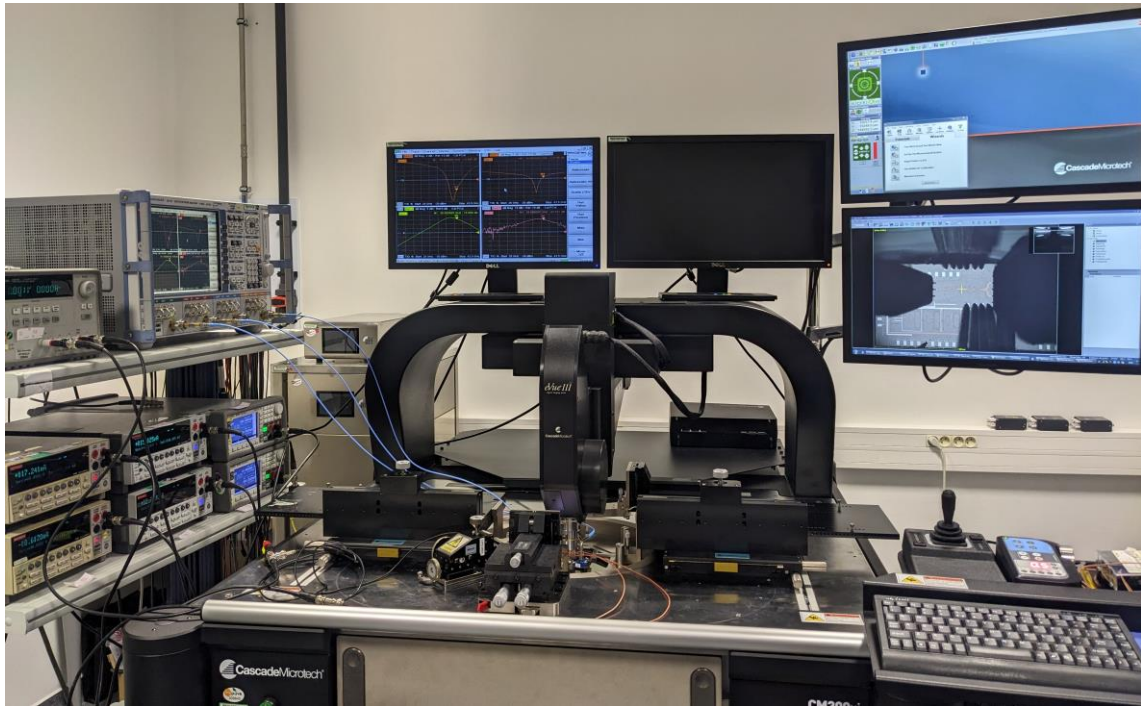
Figure 88: TESTCHIP22 PA-LNA test setup
