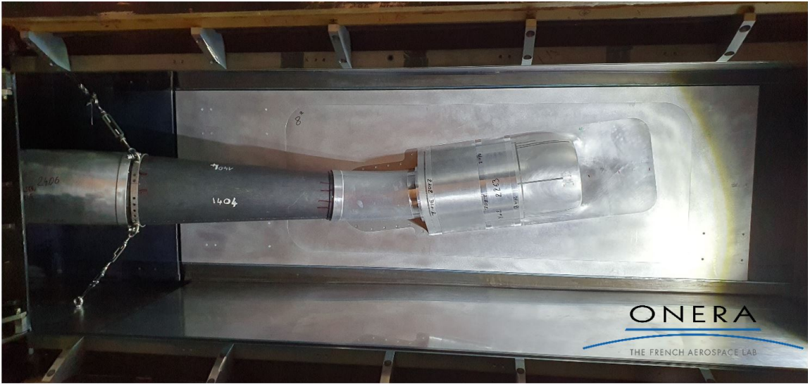
Figure 3.3: Model placed in S3Ch wind tunnel.
