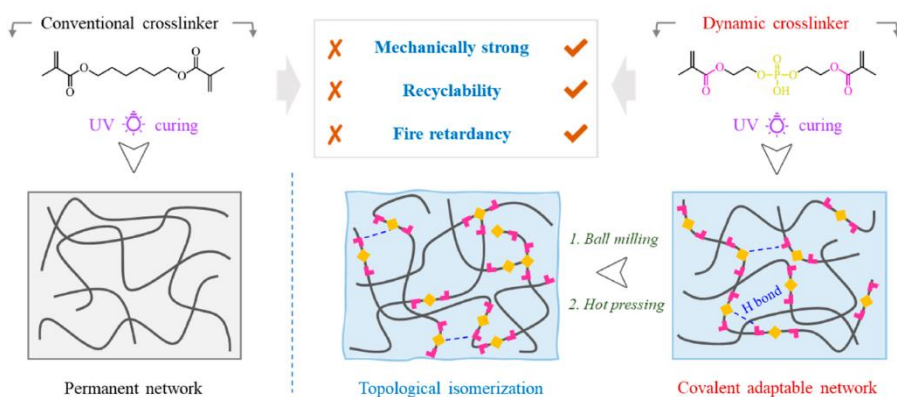
Figure 23. Performance comparison between the conventional cross-linker (HDA) and the dynamic phosphate diester-based cross-linker (PBA) 115
