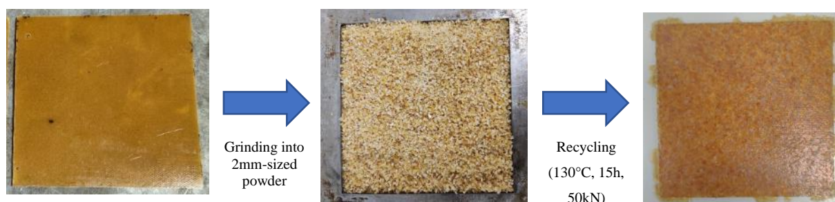
Figure 122 : Recycling of EPOXY+APP plate
