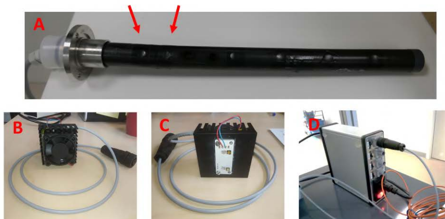
Figure 7.9: (A) shows the UV-C lamp with the arrows indicating the position of the openings on the protective tube. (B) and (C) are the back and front view of the homemade UV-C LED systems. (D) is the control unit used with the UV-C LEDs.
