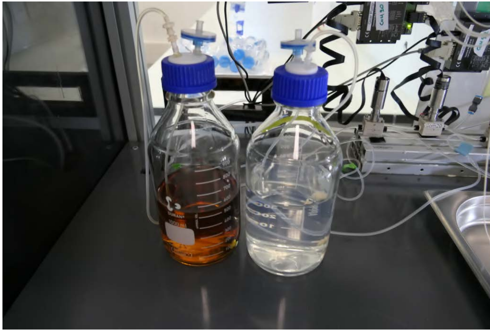
Figure 7.14: Reservoirs containing the concentrated solution of nutrients (BHI) on the left and the biocide solution (Tergazyme) on the right. The solutions were supplied into the system using a pair of gear pumps.
