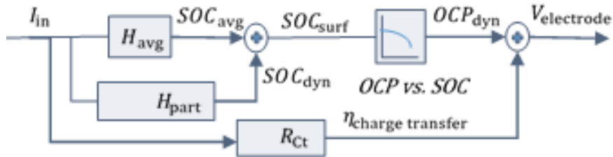
Figure 2-6 Block diagram implementation of the electrical fractional model
