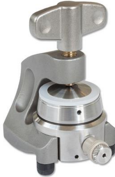
Figure 3-1 ELcell setup for potential measurement (described in - ELcell setup)
