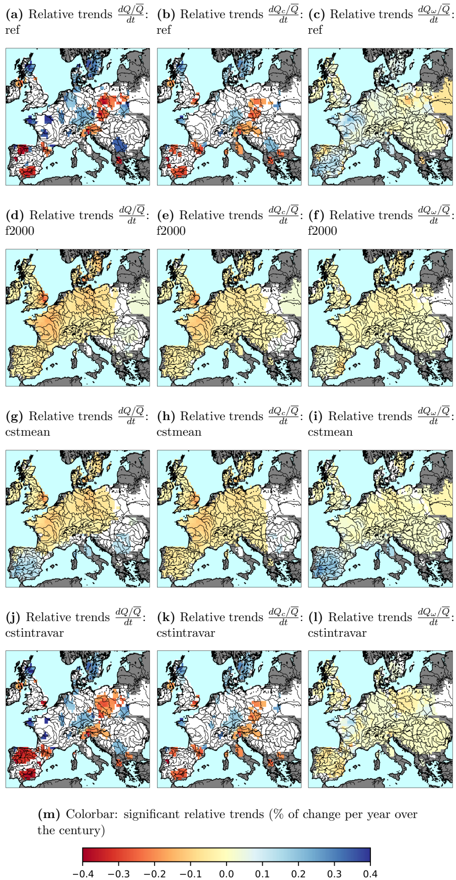
Figure 3.17 – Decomposition of significant relative annual mean discharge Q trends (% of change per year over the century) for all the tested forcings: the first line is the reference forcing. The first column is the total change in Q , the second is the partial change due to trends in the annual average of P and PET , and the last column is the partial change due to changes in the evaporation efficiency, mostly due to trends in the intra-annual distribution of P and PET . For the modified forcings: f2000 has the annual average and intra-annual distribution of P fixed for every year to their value for the year 2000. cstmean has only the annual average of P fixed. cstintravar has only the intra-annual distribution of P fixed. White areas don't have significant trends.
