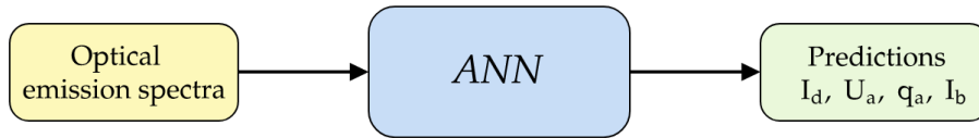
Figure 8.8: Schematic representation of the learning process for macroscopic parameters in HET. This figure illustrates the development of ANNs to predict the anode voltage U_a , discharge current I_d , anode flow rate q_a , and coil current I_b based on optical emission data.
