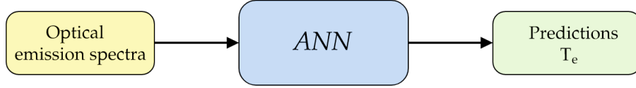
Figure 8.5: Schematic representation of the learning process for inverting the HETOD CRM. This figure illustrates the development of ANNs to predict the electron temperature T_e based on optical emission data.
