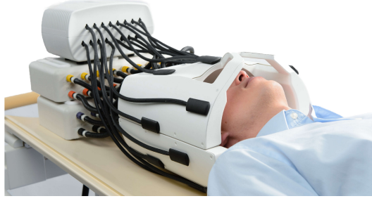
Figure 3.2: Skope Magnetic Resonance Imaging AG's field camera consisting of ^{19}\text{F} probes.
