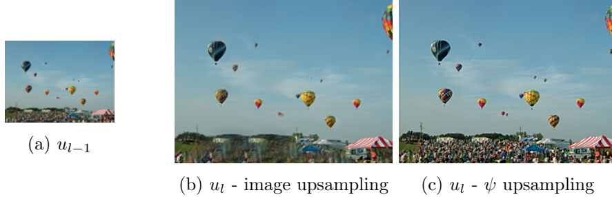
Figure III.4: For the same image at a coarser scale, the results are very different when upsampling through u or through \psi . Details are lost when using a simple bilinear upsampling of the image u (lower left).
