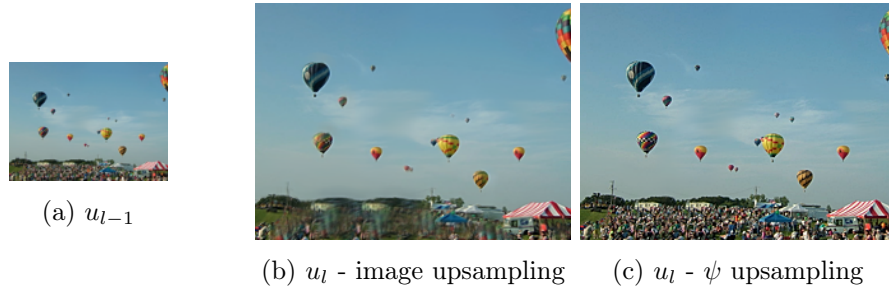
Figure III.4: For the same image at a coarser scale, the results are very different when upsampling through u or through \psi . Details are lost when using a simple bilinear upsampling of the image u (lower left).
