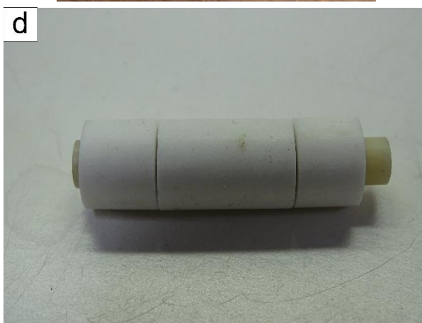
Figure VII.8. (a) The inner salt pieces are cut at the right dimensions using the diamond saw. Their length is then adjusted, and their ends plane parallelized with sandpaper. (b) Their inner diameter could be adjusted with a special grinding tool if needed. (c) The middle inner salt piece fit the jacket length. (d) The three inner salt pieces are put around the jacket and the pistons. The pistons are longer than the inner salt pieces in order to fit into the small Cu disc at the bottom (left on the image) and the big Cu disc and top lead piece at the top (right on the image).
