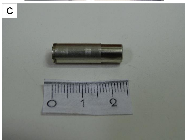
Figure VII.3. (a) One cup is first weld sealed at one extremity of the platinum tube using PUK welding machine. (b) The sample is twice wrapped into a Nickel foil. (c) The sample and the Ni foil are inserted into the half-welded jacket. The needed H_2O is added at the bottom before inserting them. (d) The second cup is weld sealed on the platinum tube. The jacket is ready.
