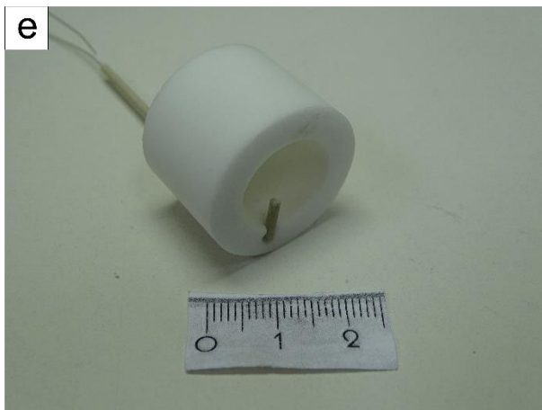
Figure VII.9. (a) The outer salt pieces are grinded with sandpaper to obtain the right length. (b) The bottom outer salt piece is drilled in order to pass the thermocouples inside. (c) The top part of the drill is dug with a scalpel to receive the 90^\circ angle of the thermocouples. (d) At the bottom part of the bottom salt piece there is a special trench that will fit the small Cu disc. (e) The thermocouples should fit well inside the trench dug at the top part of the outer bottom salt piece.
