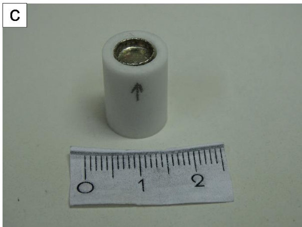
Figure VII.8. (a) The inner salt pieces are cut at the right dimensions using the diamond saw. Their length is then adjusted, and their ends plane parallelized with sandpaper. (b) Their inner diameter could be adjusted with a special grinding tool if needed. (c) The middle inner salt piece fit the jacket length. (d) The three inner salt pieces are put around the jacket and the pistons. The pistons are longer than the inner salt pieces in order to fit into the small Cu disc at the bottom (left on the image) and the big Cu disc and top lead piece at the top (right on the image).
