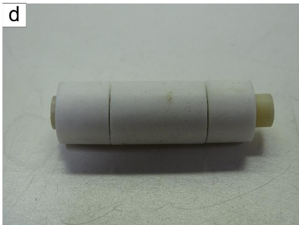
Figure VII.8. (a) The inner salt pieces are cut at the right dimensions using the diamond saw. Their length is then adjusted, and their ends plane parallelized with sandpaper. (b) Their inner diameter could be adjusted with a special grinding tool if needed. (c) The middle inner salt piece fit the jacket length. (d) The three inner salt pieces are put around the jacket and the pistons. The pistons are longer than the inner salt pieces in order to fit into the small Cu disc at the bottom (left on the image) and the big Cu disc and top lead piece at the top (right on the image).
