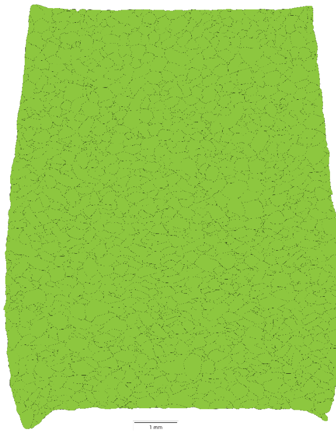
Figure VII.30. Segmentation of optical light microscopy mosaic image of deformed sample 546LN (1000 MPa) and corresponding statistics for quartzite grain sizes, aspect ratio and major axis orientation.
