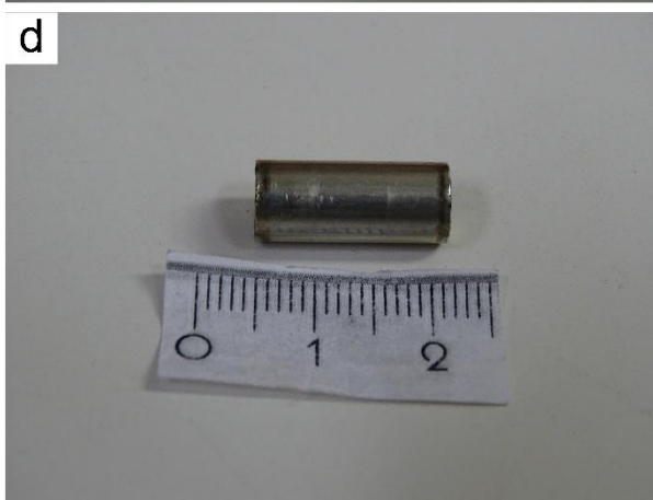
Figure VII.3. (a) One cup is first weld sealed at one extremity of the platinum tube using PUK welding machine. (b) The sample is twice wrapped into a Nickel foil. (c) The sample and the Ni foil are inserted into the half-welded jacket. The needed H_2O is added at the bottom before inserting them. (d) The second cup is weld sealed on the platinum tube. The jacket is ready.
