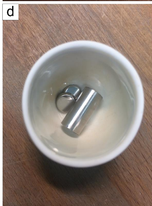
Figure VII.2. (a) Platinum tube from which the jacket is cut. (b) Two discs are cut in a platinum foil (0.15 mm) with a metal pincher (10 mm diameter). (c) The discs are then embossed with a special tool in order to form the cups. (d) The platinum tube and the two cups are then annealed at 900°C for at least 2 hours.
