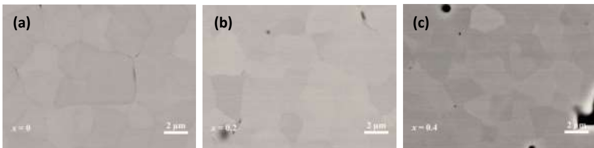
Fig 2.5 SEM (BSE) image of polished Gd_{3+x}Al_{5-x}O_{12} crystallised beads. (a) x = 0 (b) x = 0.2 (c) x = 0.4
