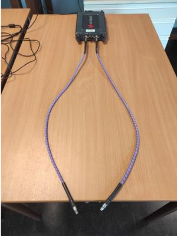
Figure 5.1 Keysight Streamline connected to the coaxial cables.
