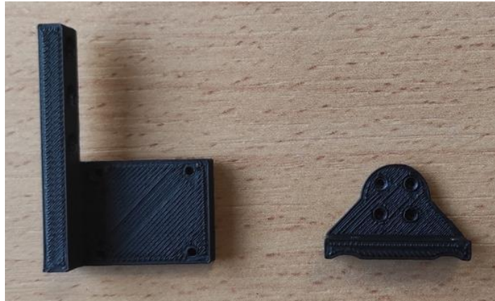
Figure 3.21 the attachment pieces 3D printed in PLA (at IEMN).
