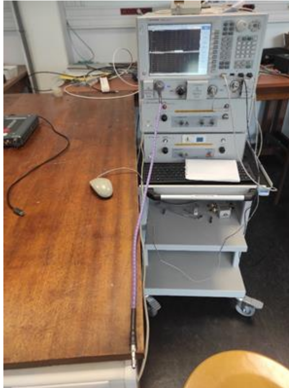
Figure 5.2 Keysight PNA connected to the coaxial cables.
