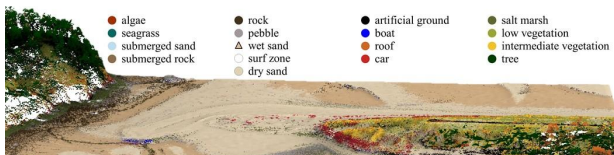
Figure 8. Extract of the resulting 3D classification: the sandy dune of Sables d’Or les Pins and its surroundings.
