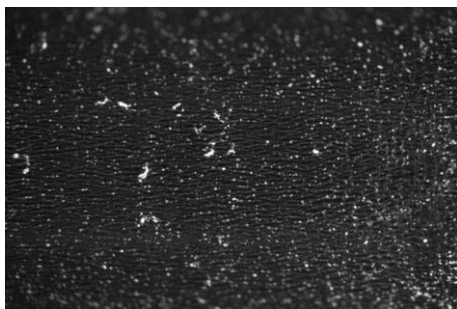
Figure 11. Micrograph of (a): NBR/PVC CB7.5 and (b): NBR/PVC G7.5 blends after 25h of irradiation (x10)
