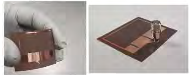
Fig. 8. Photo of the manufactured antenna in cleanroom and with U.FL connector and SMA adaptor mounted.
