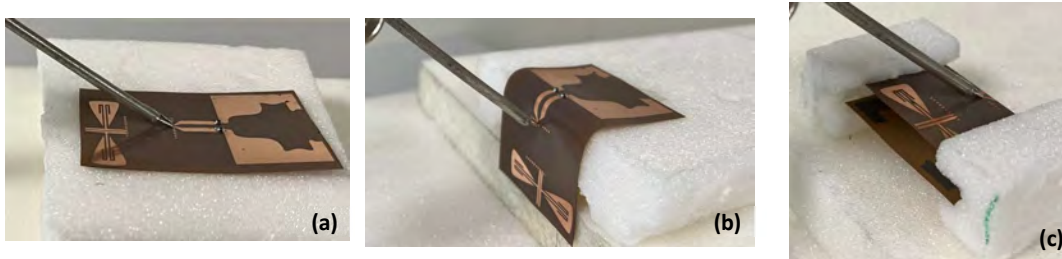
Figure V.17. Fabricated flexible antennas on polyimide substrate: (a) Flat, (b) 90^\circ Folded, (c) 180^\circ Folded.
