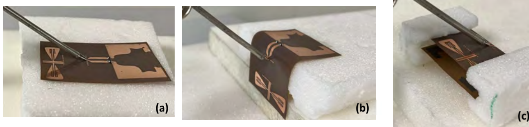
Figure V.17. Fabricated flexible antennas on polyimide substrate: (a) Flat, (b) 90^\circ Folded, (c) 180^\circ Folded.
