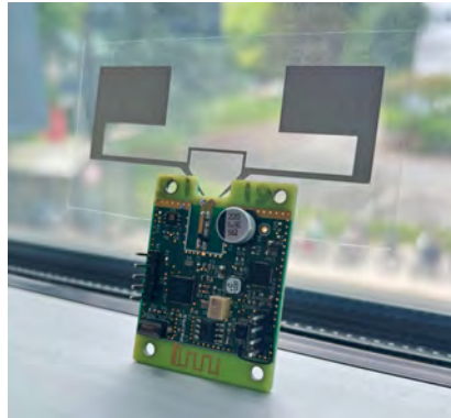
Figure III.25. Photo of the manufactured of battery-free SN prototype including a flexible antenna manufactured on transparent PET substrate operating in ISM 868 MHz frequency band.
