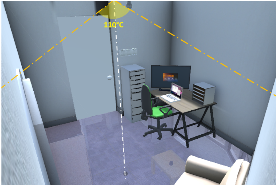
Figure 4.6 – Example of a range detection sensor (110°)
