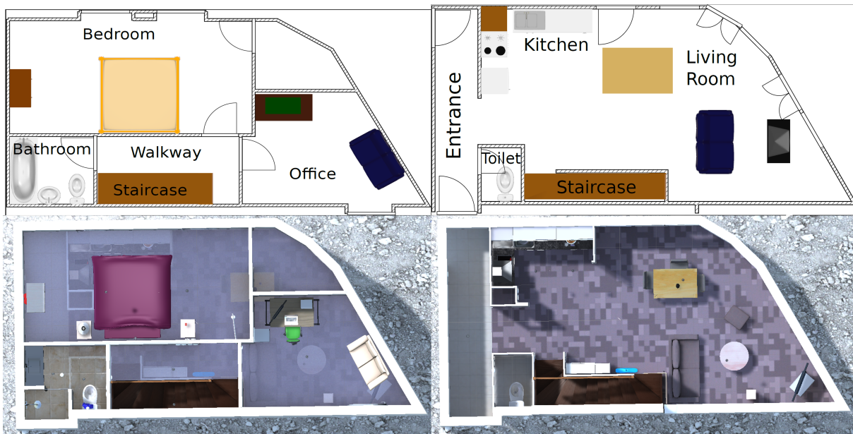
Figure 4.3 – The plan of the ground floor (left) and first floor (right) of the home used in Orange4Home and replicated in the virtual environment shown below.
