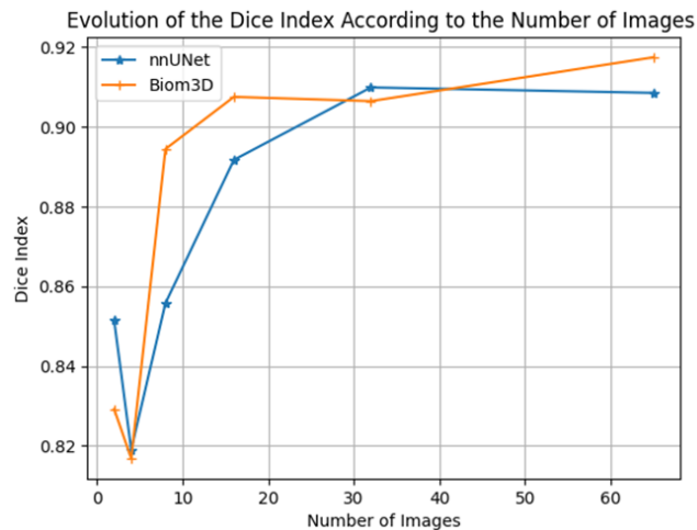
Figure 4-2 – Preliminary comparison between Biom3d (orange) and nnU-Net (blue) . The Dice scores are obtained using the same testing set while training on set training sets of increasing sizes (2, 4, 8, 16, 32 and 65 images). The curves drop down between 2 and 4 images probably due to bad annotations.
