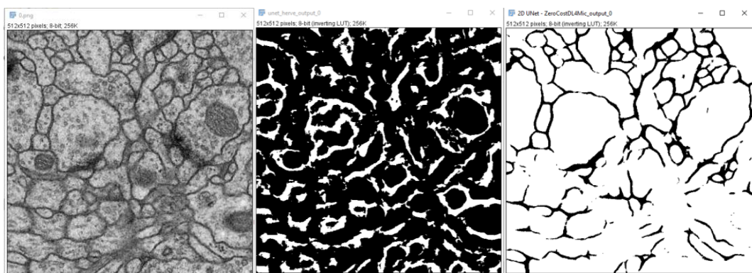
Figure 2-7 – Segmentations done with DeepImageJ of membranes captures with an electron microscope. The raw image ( left ) is segmented first by an inappropriate model ( middle ) and an appropriate model ( right ).
