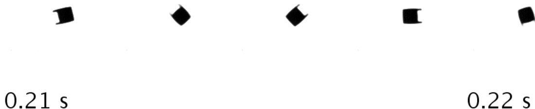
Figure 67: Capture of a full rotation achieved by generating a 140 Hz frequency rotating field from Helmholtz setup in less than 10ms.
