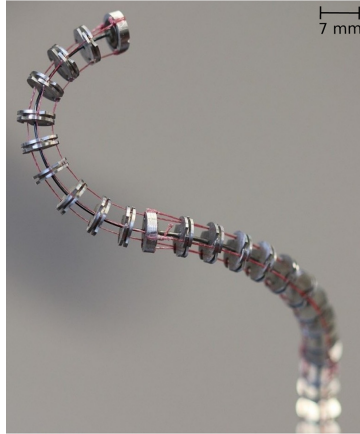
Figure 1.4: A tendon actuated continuum robot (the METABot (Magnetically Extensible TACR)) presented in [Amanov et al. 2021].
