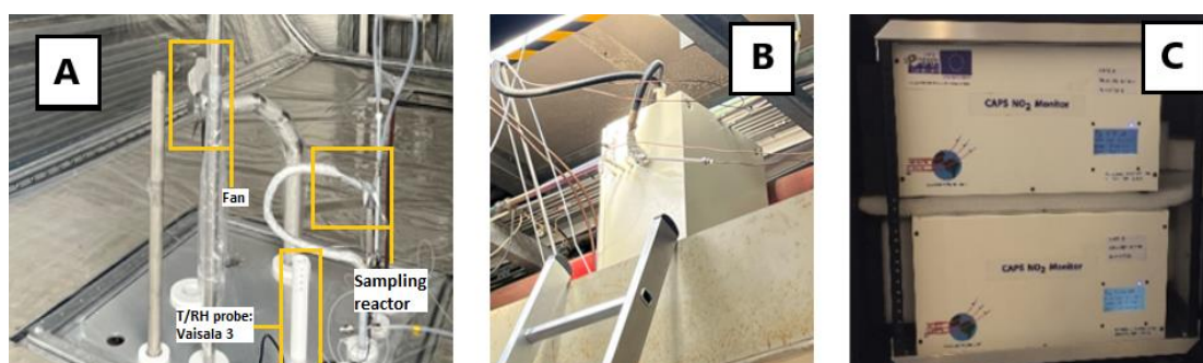
Figure 3. 4: IMT-CA coupling to SAPHIR, A- CA sampling reactors inside SAPHIR, B- CA sampling system lifted on the container's roof below the chamber's floor, C- Two \text{NO}_2 monitors housed inside the container
