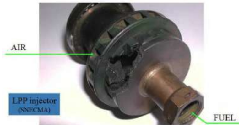
Figure 1.12. – An injector of a Safran Aircraft Engines Lean Premixed Prevaporized combustor damaged by a thermoacoustic instability. Reproduced from [53].
