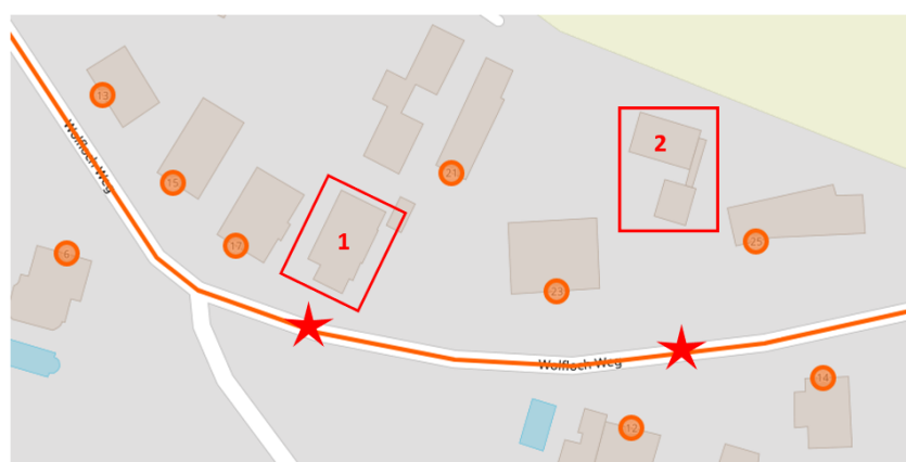
FIGURE 7.2 – Copyright OpenStreetMap (Taken the 07/03/2022) - A random street without any relation to the insurer's portfolio. Several issues can be seen. Stars correspond to address geolocation and squares to the related building. The buildings are not well reported in the building database, with no number being linked to them. Building 1 has an annex and can easily be linked to 19 Wolfloch Weg Colmar or 19 rue de WolflochWeg Colmar. Residential house 2, linked to 23 bis Wolfloch Weg Colmar, is 20 meters from the street and is composed of several buildings.
