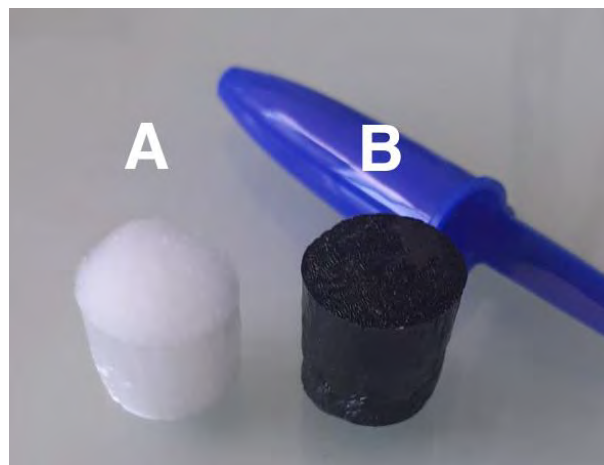
Figure 2.5 – Directional freeze-cast aerogels. Plain agarose (A) and nanocomposite (B) aerogel.
