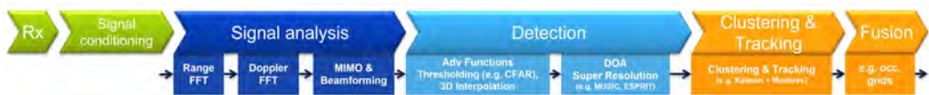
Figure 1.5: Radar signal processing chain. First, the received signal is converted from the time domain to the frequency domain to extract distance and velocity information. An object detector is applied to find the range and velocity bins where there are objects. Then, the azimuth (and the elevation) of objects is estimated. Finally, some post-processing steps are applied to output the final target list.
