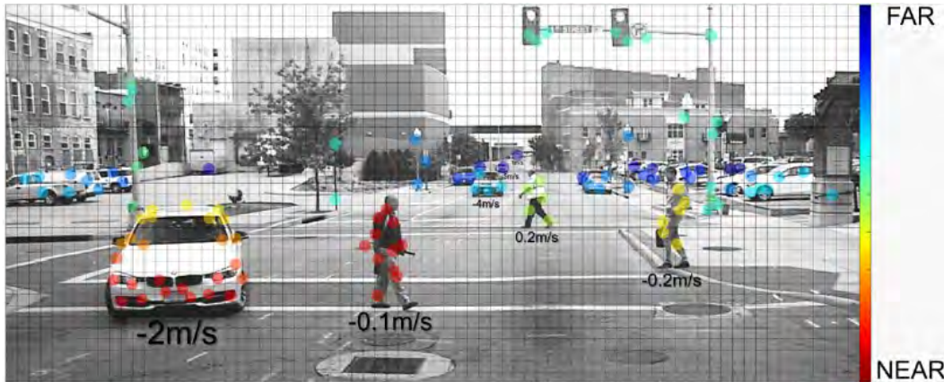
Figure 8: Example of radar point clouds. Source: [Gu 2022]
