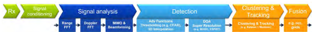
Figure 1.5: Radar signal processing chain. First, the received signal is converted from the time domain to the frequency domain to extract distance and velocity information. An object detector is applied to find the range and velocity bins where there are objects. Then, the azimuth (and the elevation) of objects is estimated. Finally, some post-processing steps are applied to output the final target list.
