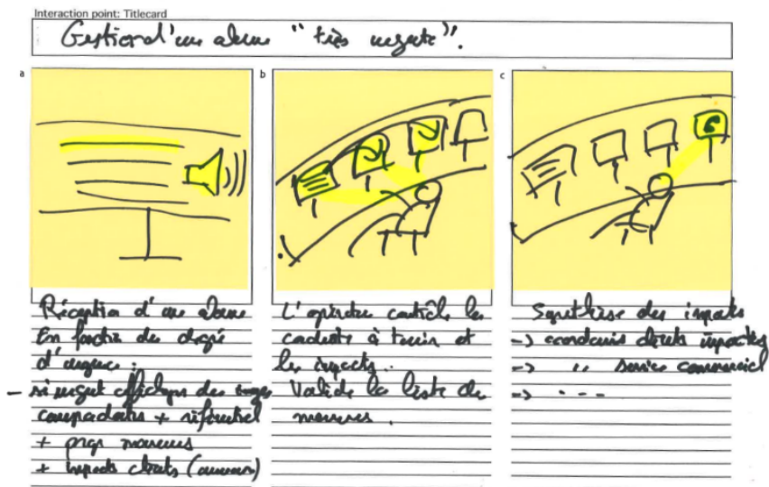
Figure 7.1. Management of a very urgent alarm: There is an urgent alarm, and the system displays all the necessary information (referential, maneuver preparation...). The operator reviews the information and validates the maneuvers. then he is presented with a summary of the impacts: the impacted customers, and the interlocutors who could be impacted.
