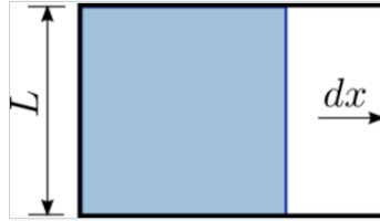
Figure 2.18 – Illustration of the force necessary to increase the surface area. dF = \gamma dx F = \gamma L for one interface.
