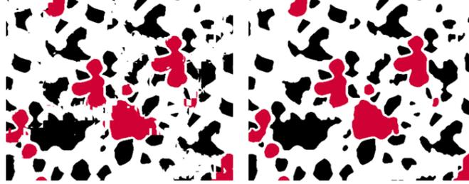
Figure 6.4 – MPS image before (Left) and after (Right) post-processing, black: solid, red: air, white: water.
