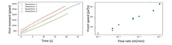
Figure 3.26 – Repeatability of the injection in saturated conditions: First moment evolution with time for a given flow rate (Q=0.01mL/min), for 4 repetitions (left); Front velocity as function of flow rate (right)
