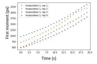
Figure 3.28 – Repeatability of the injection: First moment evolution with time for a given flow rate (Q=0.01mL/min), for 4 repetitions in unsaturated conditions.
