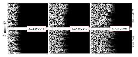
Figure 5.19 – Comparison of experimental and simulated concentration fields for three normalized times,  $S_w = 0.87$ .
