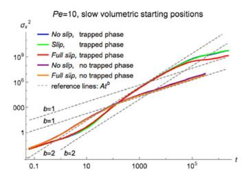
Figure 2.27 – Pore scale simulations of dispersion in saturated (no trapped phase) and unsaturated media (trapped phase). Variance as function of time, for different slip conditions. The lines b = 1 correspond to Fickian dispersion while the lines b = 2 correspond to ballistic dispersion (non Fickian). From Triadis *et al.* (2018) [157].
