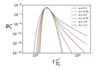
Figure 2.7 – Simulations of breakthrough curves (BC) as a function of dimensionless time  $t\frac{u^2}{D_0}$  with different levels of permeability fluctuations  $\sigma_f$ . From Talon, Ollivier-Triquet *et al.* 2023 [151].
