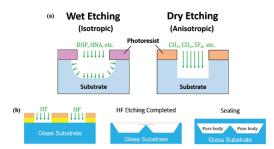
Figure 2.31 – Schematic of the etching technique, from Anbari, 2018
