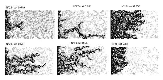
Figure 5.12 – Preferential flow paths for different saturation values. The experimental images have been binarized to emphasize on the tracer concentration flow paths.
