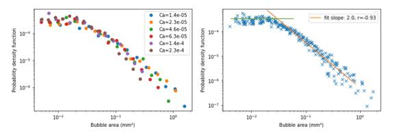
Figure 5.6 – Air bubbles probability density functions p(s). (Left) pdf of the distributions for different values of capillary numbers. (Right) pdf of all the distributions and fit with a power law  $p(s) \propto s^{-2}$ .
