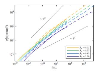
Figure 2.28 – Simulation of advective dispersion in time for four saturation values. The plot compares  $\sigma_x^2$  using the particle tracking analysis (continuous lines) with  $\sigma_x^2$  from a CTRW approach computed using the predicted velocity PDF  $p_E(v)$  (dashed lines). From A.V Parra *et al.* (2021).
