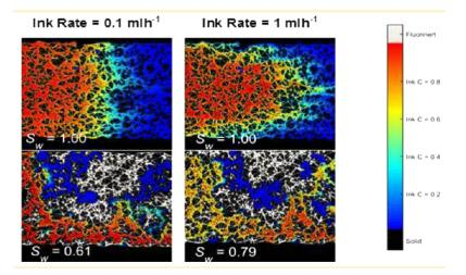
Figure 2.36 – Micromodel experiment of dispersion in unsaturated porous media, from Kadamitriou *et al.*, 2016 [93].
