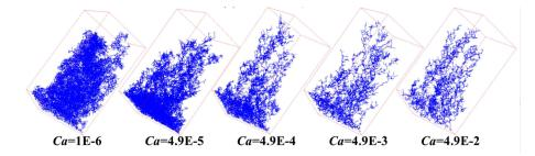
Figure 2.19 – Capillary fingering: effect of increasing Ca from left to right. Adapted from Tang (2020) [153]
