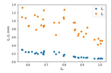
Figure 7.9 – Correlation characteristic length as a function of saturation in the transverse direction  $\xi_y$  for and in the longitudinal direction  $\xi_x$  for a threshold  $r_{\zeta} = 0.05$ .
