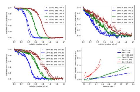
Figure 5.21 – [Top and bottom left] Comparison of experimental and simulated concentration profiles for three normalized times, and three saturation values respectively  $S_w = 1$ ,  $S_w = 0.87$  and  $S_w = 70$ . [Bottom right] Comparison of the second moment evolution with the normalised time t' for three saturations in simulation and experiments. An offset has been subtracted to the second moment for a better comparison of the slopes.
