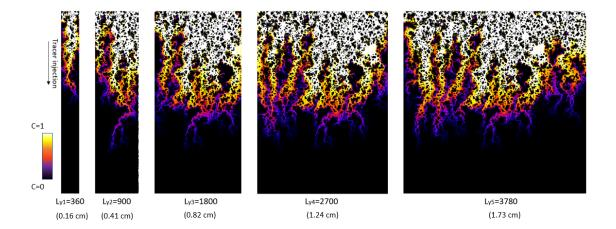
Figure 7.27 – Effect of width on the transport. Concentration fields as a function of the position x at t' = 100000 (LBM units) = 2.3s for 5 different widths.
