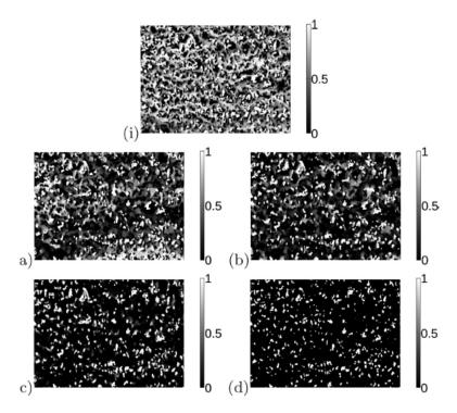
Figure 2.23 – Probability maps of trapping for different Ca numbers:  $Ca = 3.7.10^{-7}$  (a), 7.4.10<sup>-6</sup> (b), 3.0.10<sup>-5</sup> (c), and 3.3.10<sup>-4</sup> (d).
