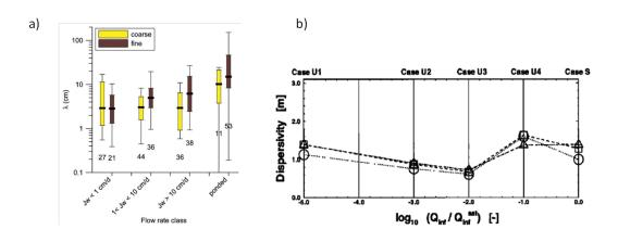
Figure 2.26 – a) Dispersivity as a function of the flow rate. From Vanderborght *et al.* (2007). b) Dispersivity as a function of the flow rate. From Birkholzer *et al.* (1997).
