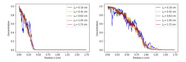
Figure 7.28 – Effect of width on the concentration profiles. Concentration profiles for 5 medium widths at t' = 30000 (LBM units) = 0.7s (Left) and t' = 100000 (LBM units) = 2.3 s (Right).  $S_w = 0.82$ .
