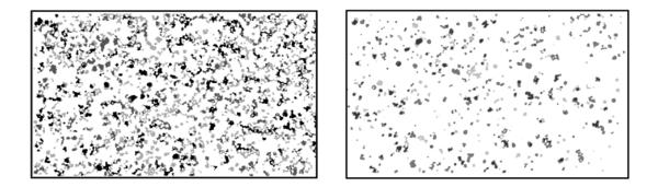
Figure 9.13 – Comparison of the bubble positions probabilities p for two Ca. (Left)  $Ca = 6.4 \times 10^{-5}$ . (Right)  $Ca = 6.4 \times 10^{-4}$ . Dark: presence of bubble for each repetition. Dark grey: p =1 Dark grey: p=0.66 Light grey: p=0.33. White: p=0.
