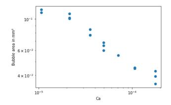
Figure 5.4 – Mean bubble area as a function of the capillary number
