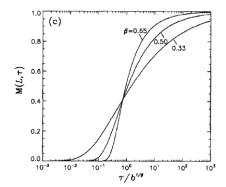
Figure 9.2 – Illustration of CFTPD (or BTC curves) with different values of  $\beta$ , with L the distance between the inlet and the outlet, and  $\tau$  a dimensionless time. The axis are normalized to allow a comparison of the curves.
