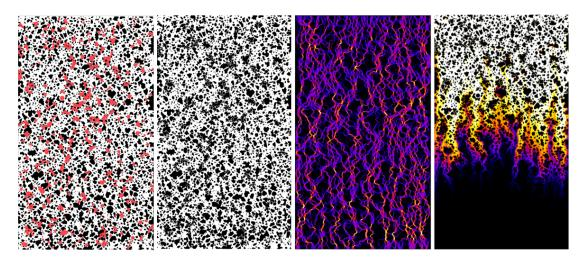
Figure 4.2 – (Left) Three phase segmented image (red: air, black: solid, white: water). [Middle left] Binary image with air clusters as solid (black) used for the velocity field simulation. [Middle right] Velocity magnitude. (Right) Concentration field for continuous injection from the top.
