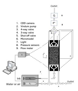
Figure 3.5 – Microfluidic set-up
