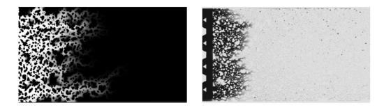
Figure 3.15 – Example of concentration fields. (Left) LBM transport simulation in saturated porous media. (Right) Laboratory experiment of dispersion in saturated porous media.
