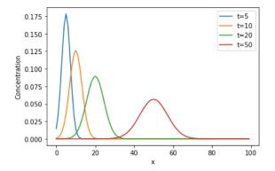
Figure 2.2 – Concentration profiles c(x,t) at different times
