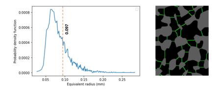
Figure 3.3 – Micromodel network characteristics, with mean values shown as dashed line. A sample of the pore network decomposition is shown on the right, throats are shown in green separating the black pores.
