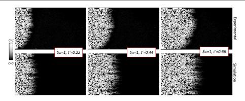
Figure 5.18 – Comparison of experimental and simulated concentration fields for three normalized times,  $S_w = 1$ .
