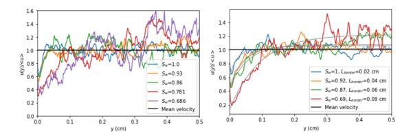
Figure 7.30 – Effect of saturation on the boundary border. Velocity profiles  $\tilde{u}^*(y)$  along the y direction (transverse to the flow) for different saturation values and medium lengths. (Left)  $L_x = 1.73$  cm (Right)  $L_x = 8.3$  cm, an exponential fit ( $\tilde{u}^*(y) = b - ae^{-\frac{y}{L_{border}}}$ ) is used to compute the border length  $L_{border}$ .
