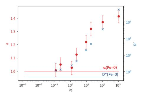
Figure 7.19 – Evolution of the power law index  $\alpha$  and the normalized dispersion coefficient  $D^*$  with the Peclet number,  $S_w = 1$ . The red and blues lines indicate the value for the simulation realized at Pe=0, for  $\alpha$  (red) and  $D^*$  (blue).
