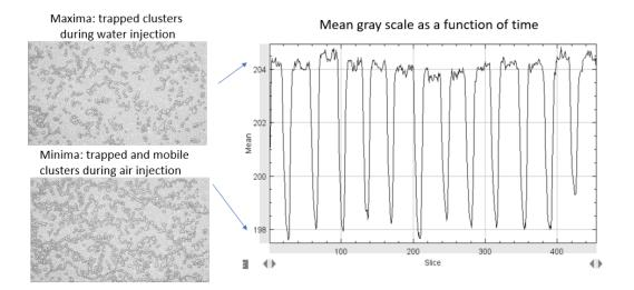
Figure 3.7 – Co-injection dynamics. (Left) unsaturated porous media during water injection with trapped air clusters (up) and during air injection with trapped and mobile air clusters (bottom). The bubbles are in darker gray. (Right) Mean gray level of the image, showing cycling behavior linked to the alternating between the water injection (trapped air clusters only) and the air injection (trapped and mobile air clusters).
