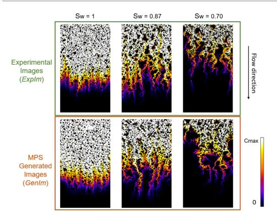
Figure 6.11 – Concentration fields simulated with Lattice Boltzmann for the three investigated saturation values for experimental images (Top) and their respective generated image (Bottom) at  $t = 1.0 \cdot 10^5$  LB units,  $c_{\text{max}} = 1$ .
