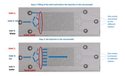
Figure 3.8 – Schematic of the injection configuration: first step
