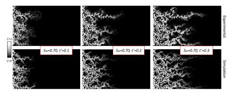
Figure 5.20 – Comparison of experimental and simulated concentration fields for three normalized times,  $S_w = 0.70$ .
