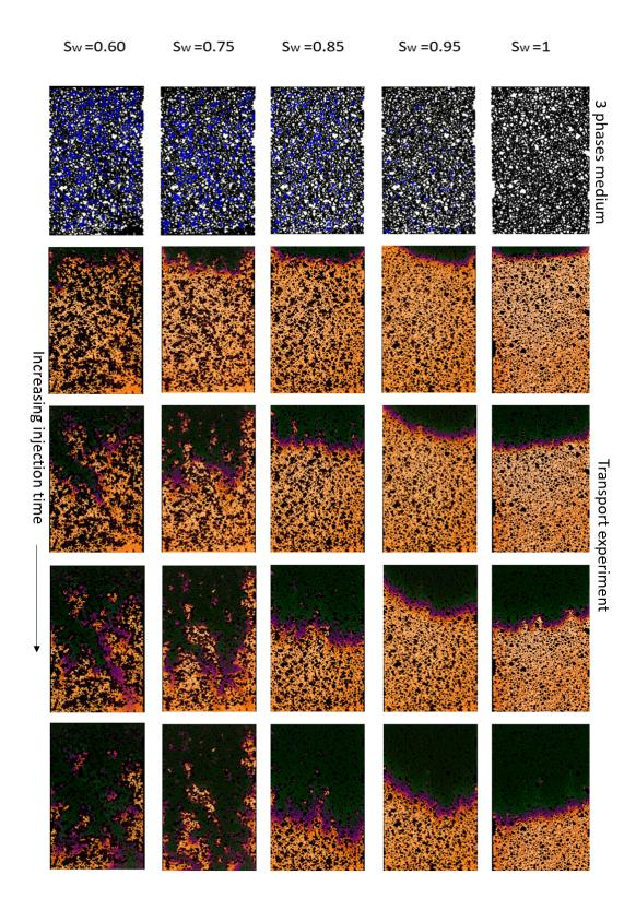
Figure 5.11 – Tracer injection experiments for 5 saturation values. First row: Phase distributions. Other columns: concentration fields. Dark green: tracer concentration. Light orange: no tracer.
