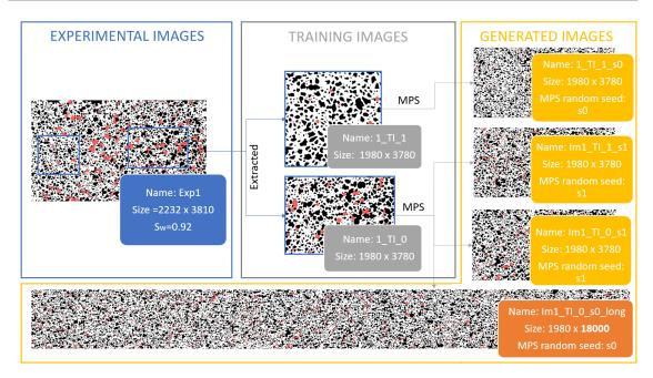
Figure 7.1 – Creation of the MPS generated images from experimental images, illustration with an experimental image of the micromodel.
