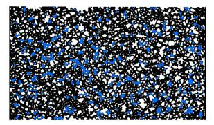
Figure 5.1 – Example of distribution after a co-injection experiment,  $Q_{water} = 0.25 \text{mL/min}$ ,  $Q_{air} = 1 \text{mL/min}$ . Black: water, white: solid, blue: air.
