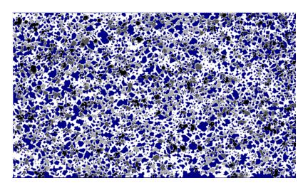
Figure 9.12 – Superposition of the bubbles positions for three co-injection experiments,  $Ca = 6.4 \times 10^{-5}$ . Blue: Solid. Dark: presence of bubble for each repetition. Dark grey: Presence of bubble for two out of three repetition. Light grey: Presence of bubble for only one repetition. White: Absence of bubble
