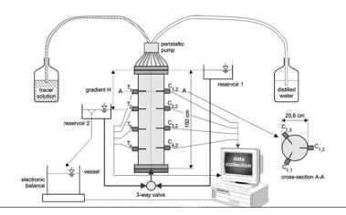
Figure 2.8 - Experimental conditions with concentration measurement at different depths, from Nützmann*et al.*(2002)
