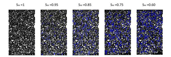
Figure 5.2 – Different saturation obtained with co-injection. Black: water; white: solid; Blue: air.
