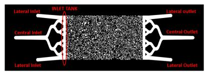
Figure 3.2 – Micromodel connectors configuration: three inlets and three outlets, an inlet and outlet tank
