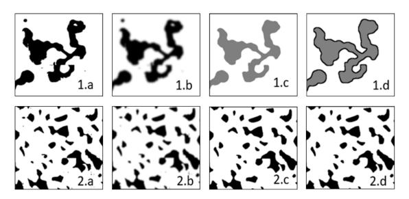
Figure 6.3 – MPS image post-processing. [Up] Air clusters processing. 1.a Air clusters before post-processing. 1.b Smoothed image of 1.a. 1.c Smoothed air clusters (binarized image of 1.b). 1.d Final air clusters image. Creation of the water film (black) around the air cluster. [Bottom] 2.a Solid grains before post-processing. 1.b Smoothed image of 2.a. 2.c Smoothed solid grains (binarized image of 2.b). 2.d Final solid grains image.
