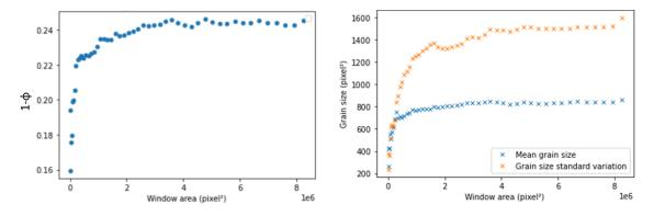
Figure 3.25 – REV of the porous media. (Left) Porosity  $\phi$  as a function of the window's size. (Right) Mean grain size and grain size standard deviation as a function of the window's size.
