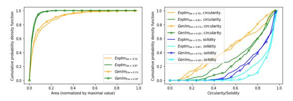
Figure 6.8 – Different distributions characterizing the shape of the air clusters for experimental images for two saturation values  $(ExpIm_{Sw=0.70} \text{ and } ExpIm_{Sw=0.87})$  and their respective MPS generated images  $(GenIm_{Sw=0.65} \text{ and } GenIm_{Sw=0.85})$ . The distributions are described through cumulative probability distribution functions. (Left) Distribution in size. (Right) Distribution in solidity and circularity.
