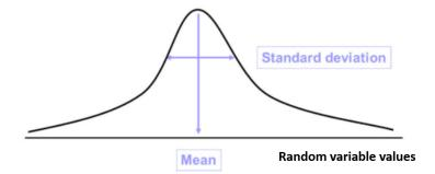
Figure 3.17 – Illustration of the first and second moment: mean position and width of the distribution
