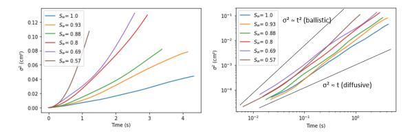
Figure 7.14 – Influence of saturation on dispersion: second moment as a function of time for different saturation values, Pe=100. (Left) Linear scale. (Right) Logarithmic scale.
