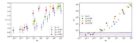
Figure 7.20 – (Left) For different saturations, evolution of the power law index  $\alpha$  with the Peclet number. (Right) For different saturations, evolution of the normalized dispersion coefficient  $D^*$  with the Peclet number. The continuous lines show values of  $D^*(Pe = 0)$  obtained from simulations with no flow.
