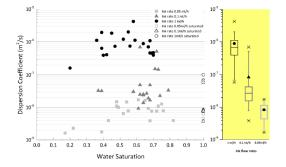
Figure 2.37 – Dispersion coefficients computed from micromodel experiments, from Kadamitriou *et al.*, 2016 [93].
