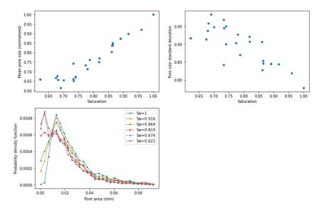
Figure 9.17 – Pore area analysis of the unsaturated networks. [Top] Mean pore size and standard variation of the unsaturated network normalized by the mean pore size in the saturated medium. [Bottom left] Distributions of the pore areas for different saturation values.
