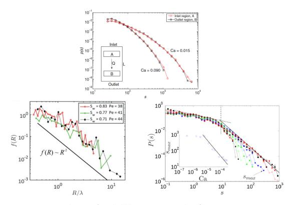
Figure 2.22 – Distribution of air bubbles in porous media after a air-water co-injection, From Jimenez-Martinez *et al.* [91] (left), Chevalier *et al.* [35] (Right), Tallakstad *et al.* [150] (top).
