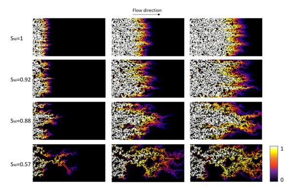
Figure 7.10 – Effect of saturation on transport. Concentration fields for 4 saturations values and three mean positions of the concentration front ( $\mu_0 = 0.18L_x$ ,  $\mu_1 = 0.43L_x$ ,  $\mu_2 = 0.65L_x$ ).
