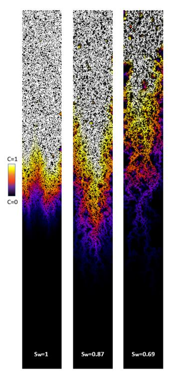
Figure 7.11 – Effect of saturation on long time dispersion. Concentration fields for 3 saturations values, the concentration has been normalized by the tracer concentration.
