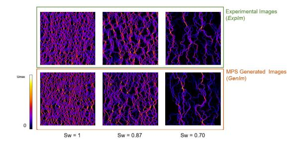
Figure 6.9 – Velocity magnitude computed with LBM (cropped images), in the experimental images [Top] and in the corresponding generated images [Bottom] for three saturation values ( $S_w = 1, S_w = 0.87, S_w = 0.70$ )  $\langle ||\mathbf{u}|| \rangle_{max} = 0.06$  (LBM units).
