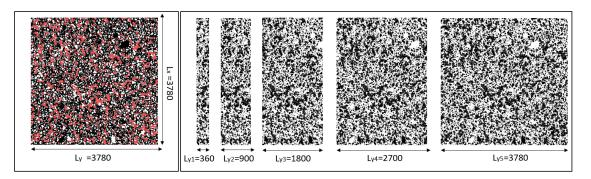
Figure 7.24 – Set of images created to study the effect of the width. (Left) Unsaturated image generated with the MPS algorithm. White: grains. Red: gas. Black: water. (Right) Images extracted from the MPS generated image width different widths  $L_y$ , indicated in pixels. Images have been binarized to compute the flow with LBM. Black: solid. White: Void.
