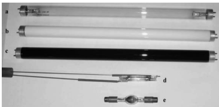
Figure 1-14: Lamps used for photochemical syntheses
