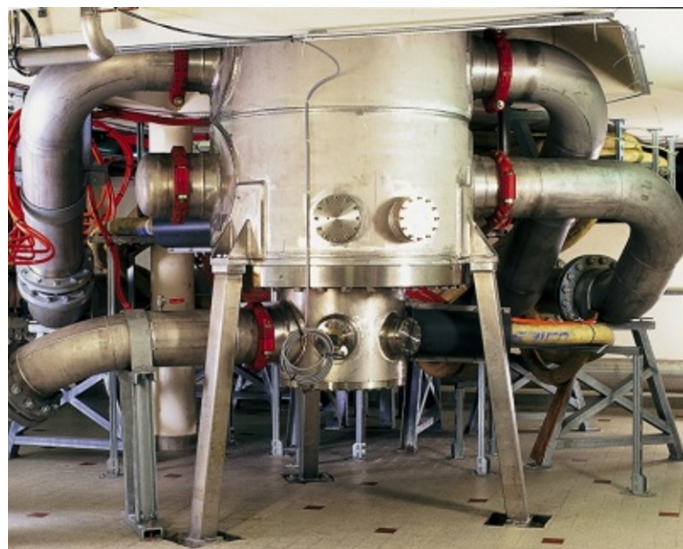
Figure 3.1: General view of the LNCMI Grenoble M9 resistive magnet: B_{max} = 37\text{ T} at I = 4 \times 15000\text{ A} . The height of the structure is approximately 2 m. The metal tubes are the water cooling: 300 l/s at \Delta p = 20\text{ bar} . The access to the magnet for user experiments is located in the floor above. Details can be found in the text and in references [25–27].
