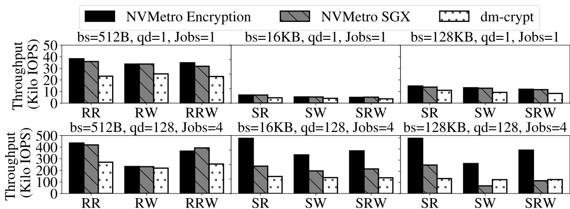
Figure 5.7: Disk encryption evaluations with fio .
