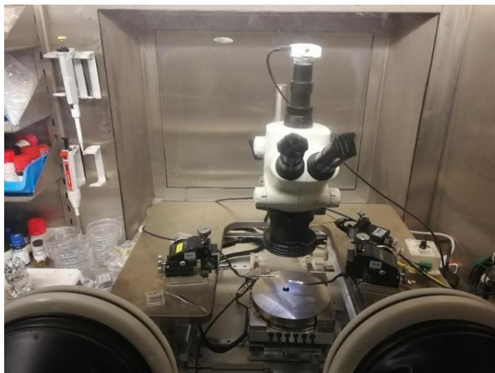
**Figure 4.15** A probe station photo in the glovebox.
