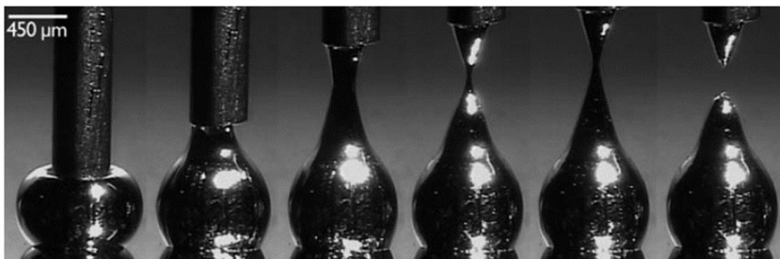
**Figure 4.12** Sequential photographs showing the formation of the EGaIn tip.<sup>[34]</sup>
